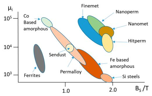
Figure 1. Permeability versus magnetic flux density of several families of soft magnetic alloys.
