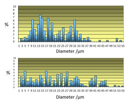
Figure 3. Particle size distribution of alloys A (up) and B (down) milled for 50 h.
