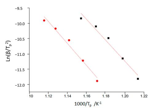
**Figure 6.** Kissinger plot of the milled alloys A (black) and B (red).
