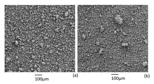
Figure 2. SEM micrographs of alloys A (a) and B (b) milled for 50 h.
