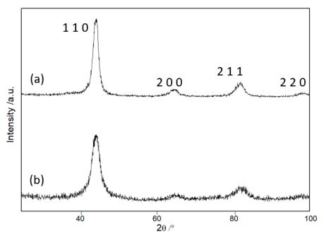
**Figure 4.** X-Ray diffraction pattern of alloys A (**a**) and B (**b**) milled for 50 h, indicating the Miller indexes of the bcc structure.
