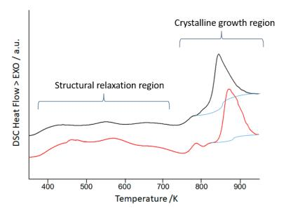
**Figure 5.** DSC scans at 10 K/min of the as milled alloys A (black) and B (red), indicating the structural relaxation and crystalline growth intervals, as well as the baseline of the main crystallisation process in both samples (blue lines).
