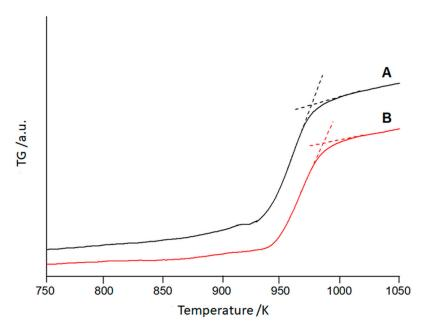
Figure 8. Magnetic thermogravimetry curves of alloys the as milled alloys A (black) and B (red).
