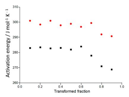
**Figure 7.** The activation energy as a function of the transformed fraction of the milled alloys A (black) and B (red).
