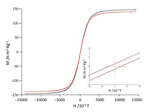
**Figure 9.** Magnetic hysteresis loops at room temperature of the milled alloys A (black) and B (red). The inset corresponds to the (0,0) region.
