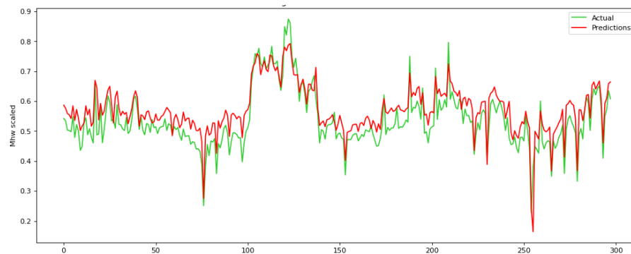
Figure 9. Actual ground truth values against the predicted ones during the training process for a parameter time step equal to 48 for the proposed RNN.
