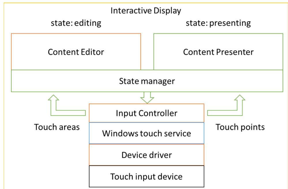
**Figure 2.** System architecture.
