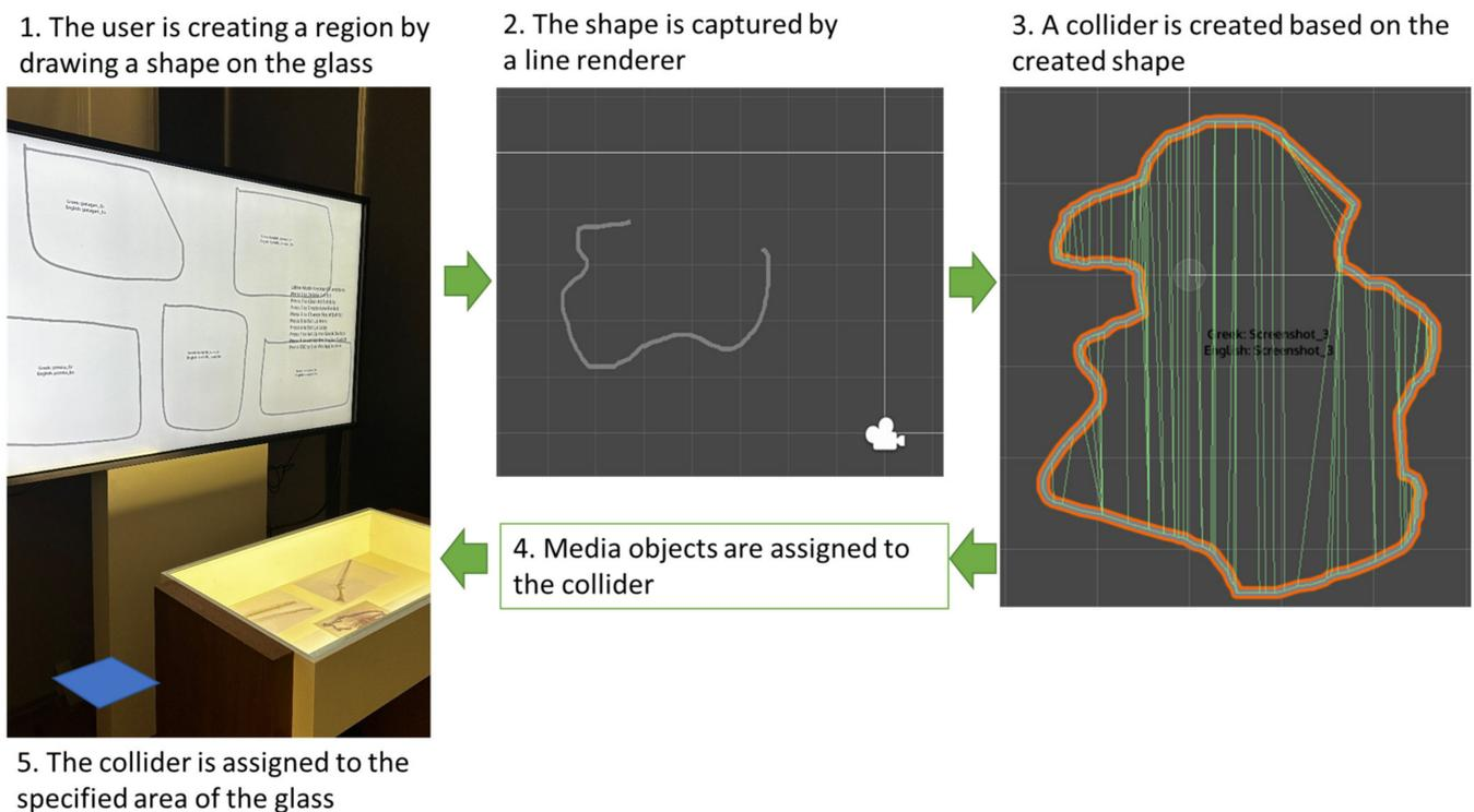
**Figure 3.** The user is touching the glass display to create an interaction area and Unity translates touch inputs to a line segment which is used to create a mesh collider which is assigned by the user with multimedia content.
