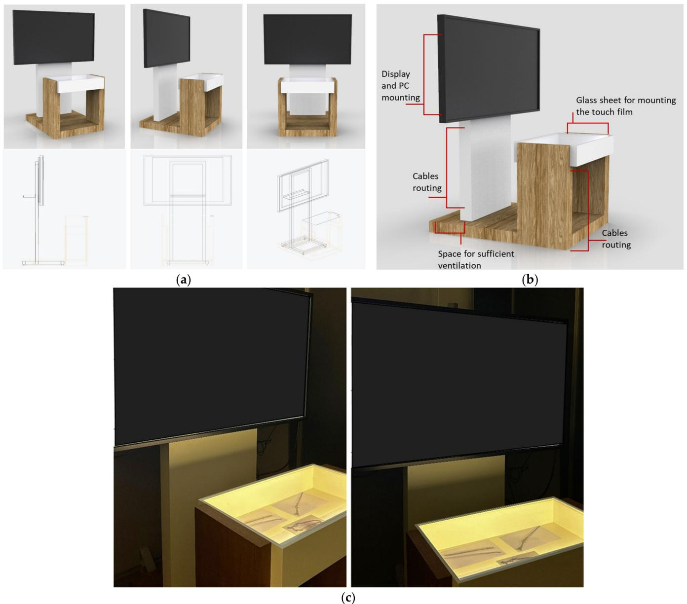
**Figure 1.** Display design (a) photorealistic and wireframe renderings; (b) analysis of negative space of the display case where equipment is integrated; (c) implementation of the prototype.
