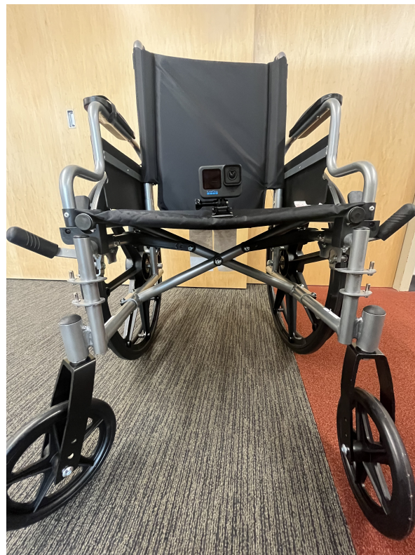
Figure 2. The configuration used for the experiments consists of a GoPro HERO10 camera mounted on the seat of the manual wheelchair.
