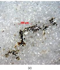
**Figure 6.** The preliminary testing results of the electrical discharge machining of samples with a sandwich-type mono-layer coating "silver + copper" after an hour of tempering at a temperature of 160 °C: (**a**) a sample after preliminary testing; (**b**) optical microscopy of the formed texture before coating removal,  $10 \times$ ; (**c**) optical microscopy of the formed texture,  $10 \times$ .
