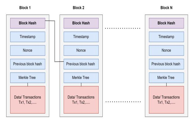
Figure 4. Structure of the blocks in Blockchain.
