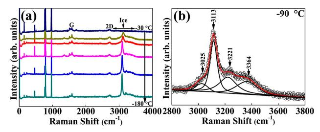
**Figure 3.** (a) Temperature-dependent Raman spectra obtained by focusing the laser to a frozen water droplet (b) fitting of the water-related peak obtained at -90 °C.
