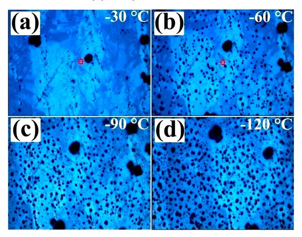
**Figure 1.** Optical microscopy images of the epitaxial graphene at (**a**) -30 °C, (**b**) -60 °C, (**c**) -90 °C, and (**d**) -120 °C temperatures.
