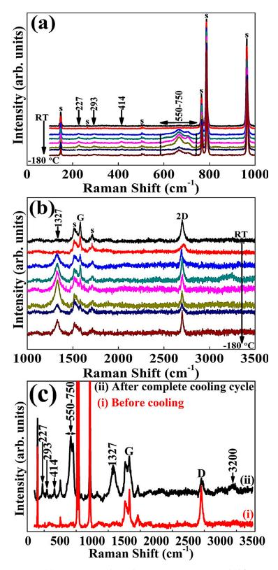
**Figure 2.** (a) Temperature-dependent Raman spectra recorded from room temperature to  $-180 \,^{\circ}\text{C}$  in Raman frequency range of 1000–3500 cm<sup>-1</sup>. (b) Temperature-dependent Raman spectra were recorded from room temperature to  $-180 \,^{\circ}\text{C}$  in the Raman frequency range of 100–1000 cm<sup>-1</sup>. (c) Raman spectra of epitaxial graphene were taken at room temperature before and after the cooling cycle.
