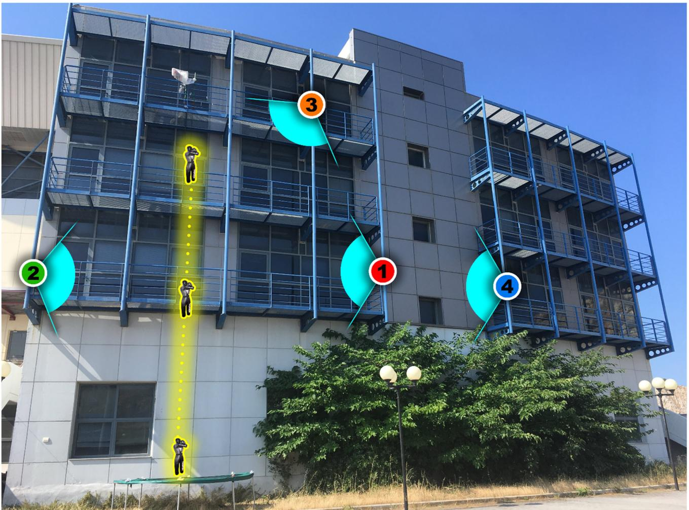
**Figure 6.** The four different locations of the building (red, green, orange, and blue) where the RGB camera was placed throughout the data acquisition process regarding the freefall (yellow) of the human dummy (as presented in [15]).
