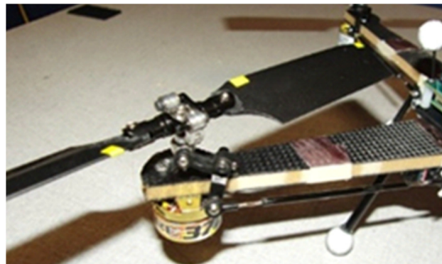
Figure 17. UAVs with variable pitch propellers [57].
