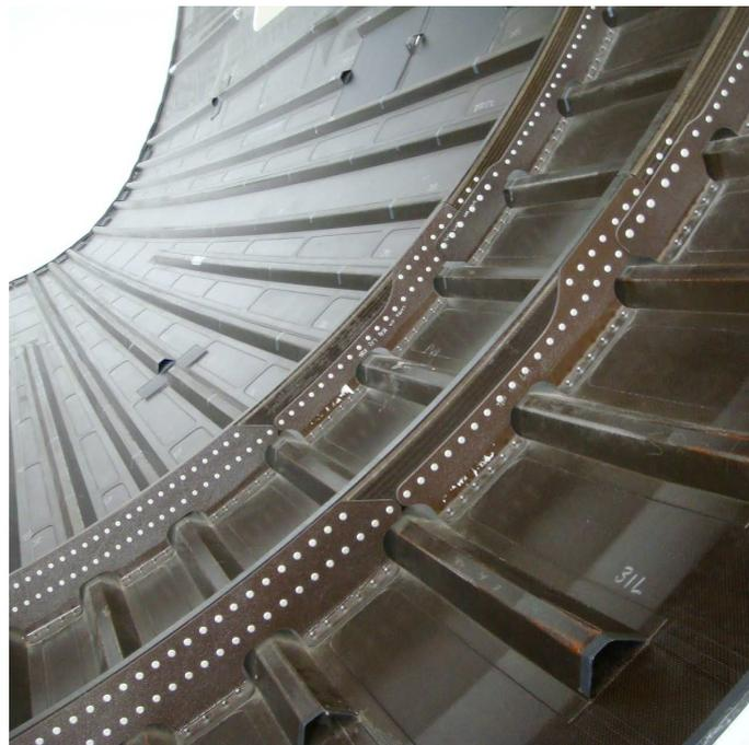
**Figure 1.** Curved panel with unconventional stringers (Boeing 787).
