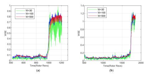
**Figure 4.** The effect of sliding window width selection on wavelet singular spectral entropy: (a) Wavelet singular spectral entropy at 2500 rpm; (b) Wavelet singular spectral entropy at 3000 rpm.
