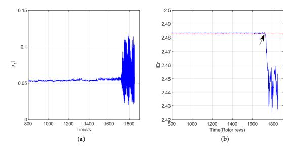
**Figure 9.** Information entropy of the spatial mode at 3000 rpm: (**a**) First-order space mode; (**b**) Information entropy.
