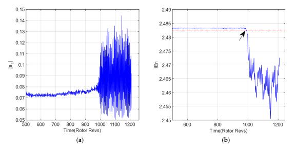
**Figure 8.** Information entropy of the spatial mode at 2500 rpm: (**a**) First-order space mode; (**b**) Information entropy.
