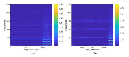
**Figure 3.** Time-frequency diagram of the first-order spatial mode: (**a**) Diagram at 2500 rpm; (**b**) Diagram at 3000 rpm.
