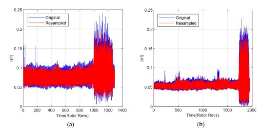
**Figure 2.** Amplitudes of spatial mode with pre-sampling and post-sampling: (**a**) Amplitudes at 2500 rpm; (**b**) Amplitudes at 3000 rpm.
