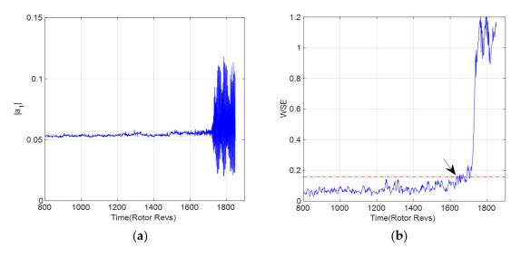
**Figure 7.** Wavelet singular spectral entropy of the spatial mode at 3000 rpm: (**a**) First-order space mode; (**b**) Wavelet singular spectral entropy.
