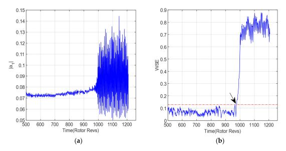
**Figure 6.** Wavelet singular spectral entropy of the spatial mode at 2500 rpm: (**a**) First-order space mode; (**b**) Wavelet singular spectral entropy.
