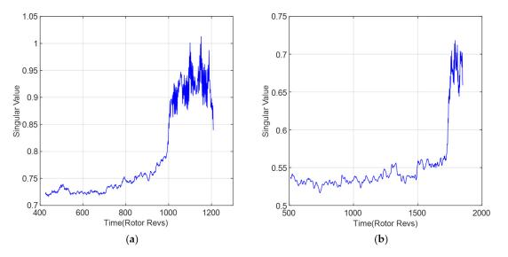
**Figure 5.** Variation of singular value in sliding window: (**a**) Singular value at 2500 rpm; (**b**) Singular value at 3000 rpm.
