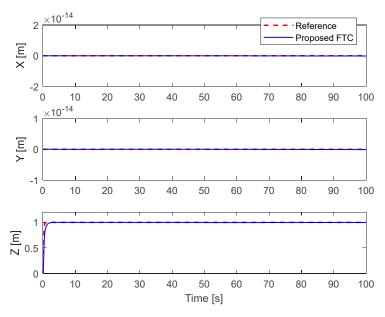
Figure 8. Altitude and position performance with simultaneous fault.
