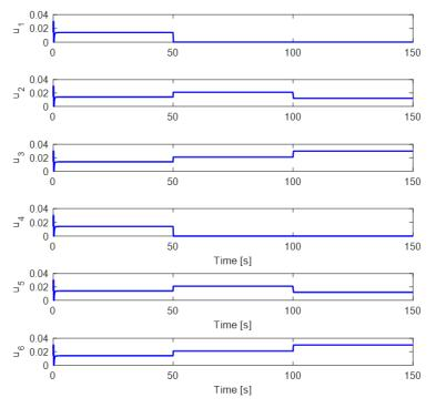
**Figure 7.** Response of motor's command with complete fault in actuator 1 and partial fault in actuator 2.
