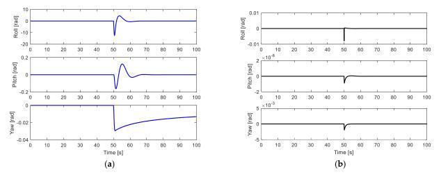
Figure 3. Attitude angle performance with 50% LoCE in actuator #2: (a) ASMC; (b) Proposed FTC.
