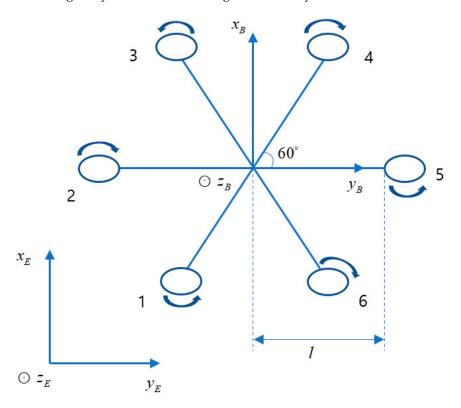
Figure 1. Hexacopter in body and inertial frames.
