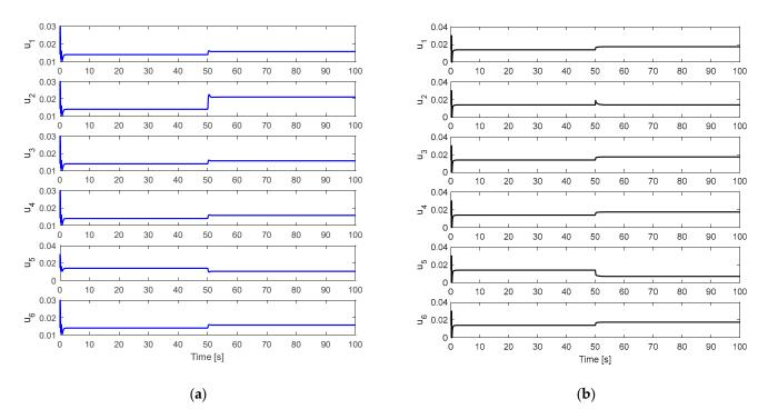
Figure 4. Response of motor's command with 50% LoCE in actuator #2: (a) ASMC; (b) Proposed FTC.
