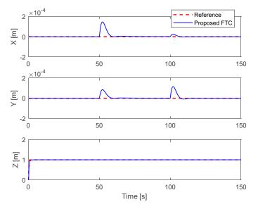
**Figure 5.** Altitude and position performance with complete fault in actuator 1 and partial fault in actuator 2.
