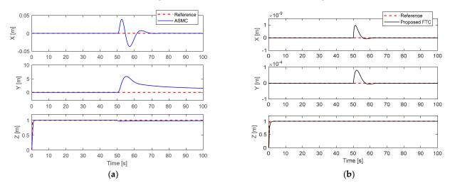
Figure 2. Altitude and position performance with 50% LoCE in actuator #2: (a) ASMC; (b) Proposed FTC.
