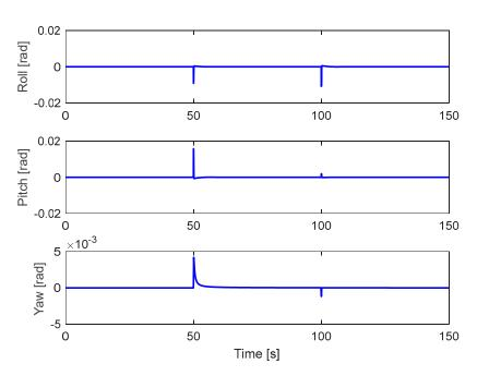
Figure 6. Attitude angle performance with complete fault in actuator 1 and partial fault in actuator 2.
