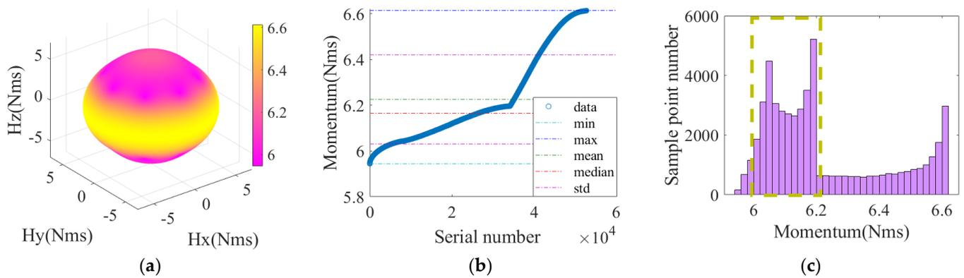
**Figure 3.** Momentum characteristics of 8-SGCMGs. (a) Momentum envelope, (b) Sample arrangement, (c) Sample number statistics.
