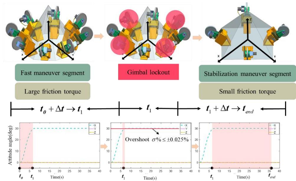
Figure 9. Reconfiguration of 8-SGCMGs into 4-SGCMGs.
