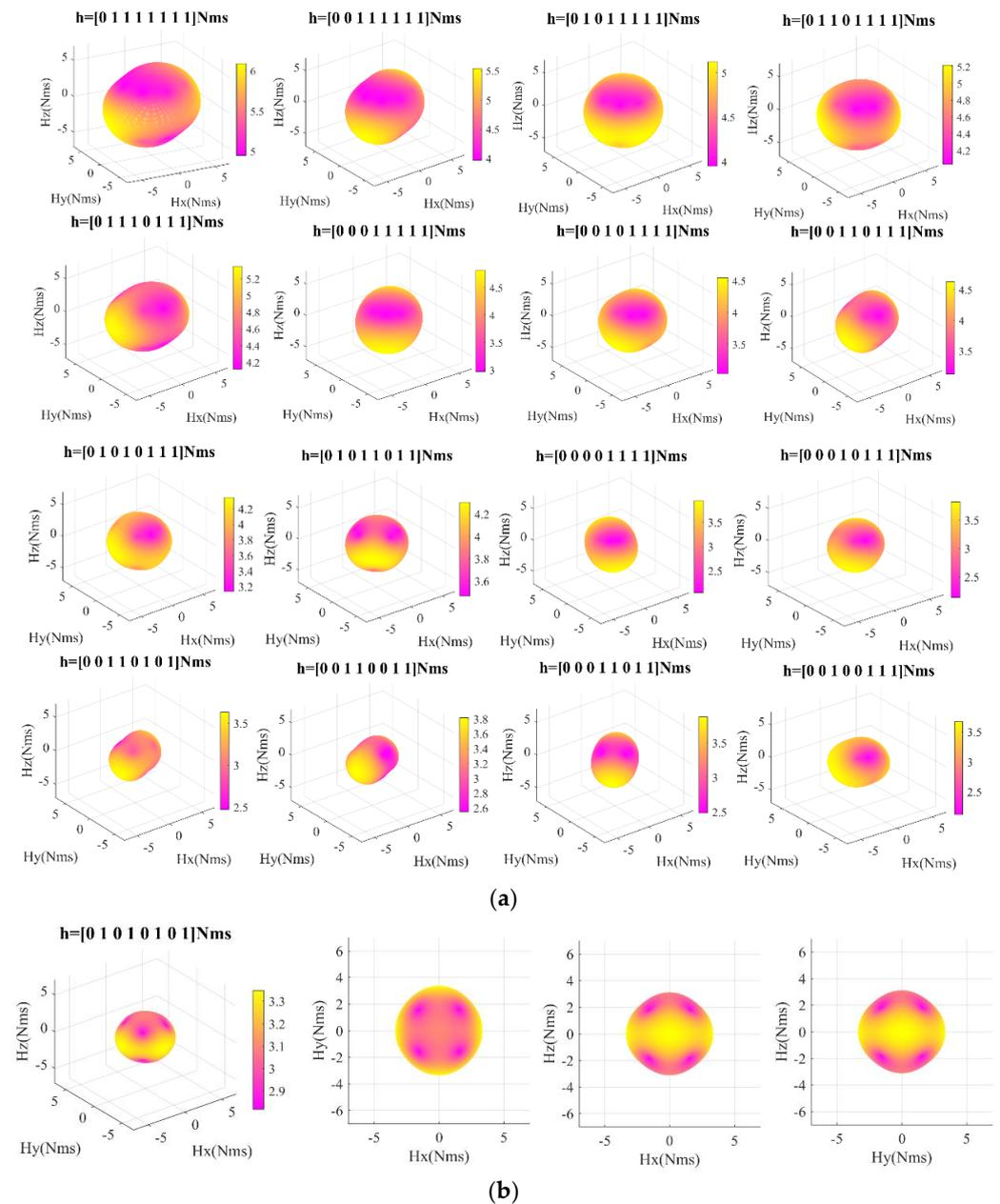
**Figure 4.** Failure momentum envelopes of 8-SGCMGs. (a) Asymmetric failure, (b) Symmetric failure.
