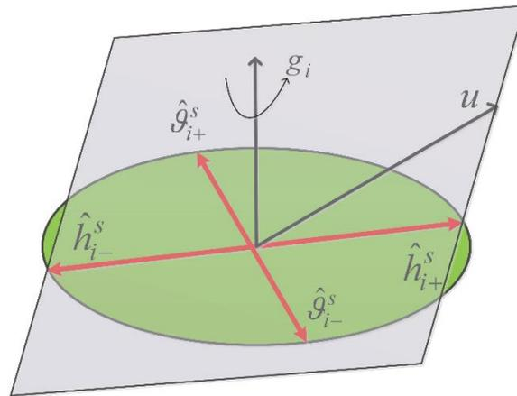
Figure 5. Singularity schematic diagram of the SGCMGs.
