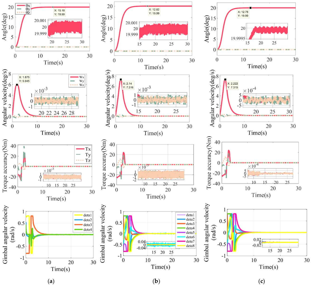
**Figure 10.** Simulation results of small-angle attitude maneuver. (a) Large 4-SGCMGs, (b) 8-SGCMGs, (c) Reconfiguration of 8-SGCMGs into 4-SGCMGs.
