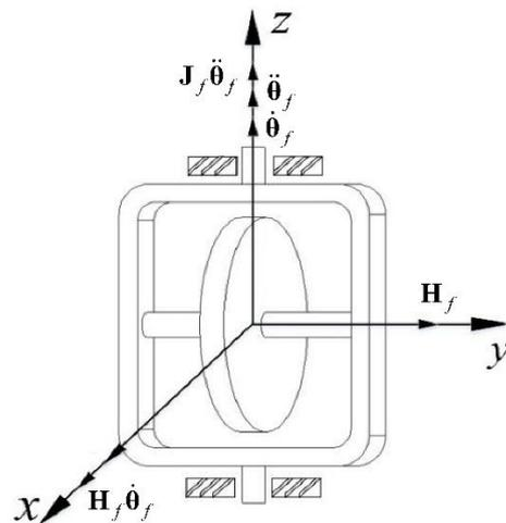
Figure 7. Schematic diagram of SGCMG system.
