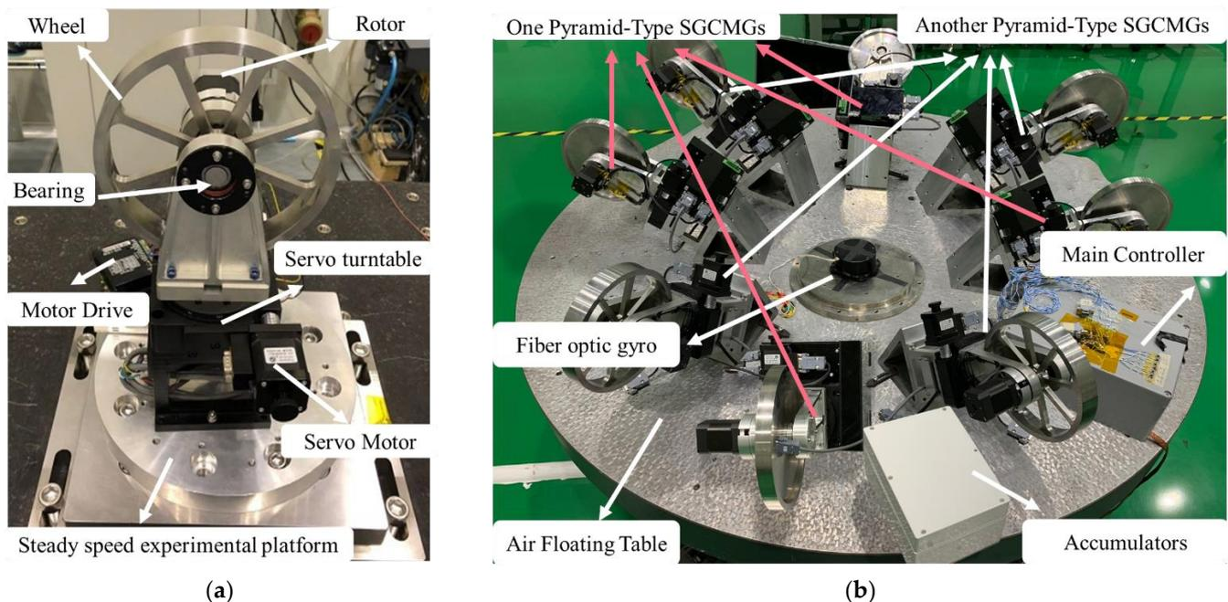
**Figure 8.** Experimental setup. (a) SGCMG prototype, (b) Octagonal cone-type SGCMGs.
