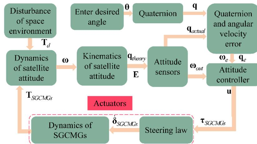
Figure 1. Attitude control system of hyper-agile satellites.
