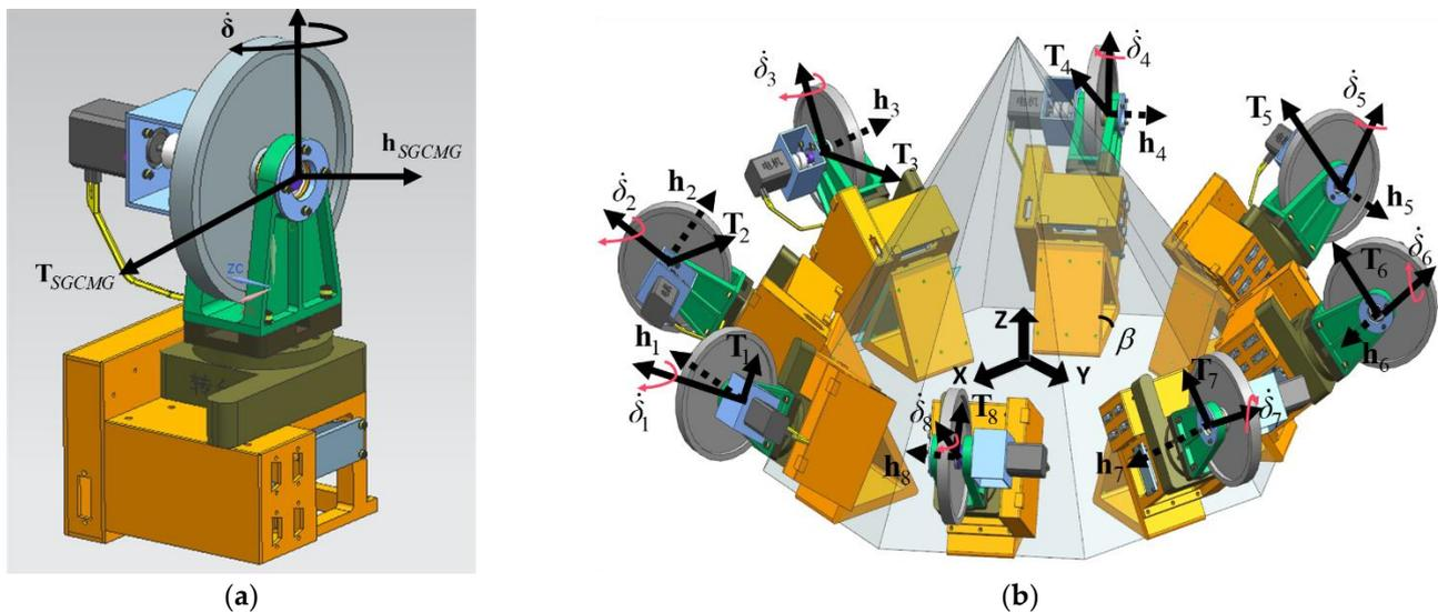
Figure 2. Composition schematic of SGCMG and 8-SGCMGs. (a) SGCMG, (b) 8-SGCMGs.
