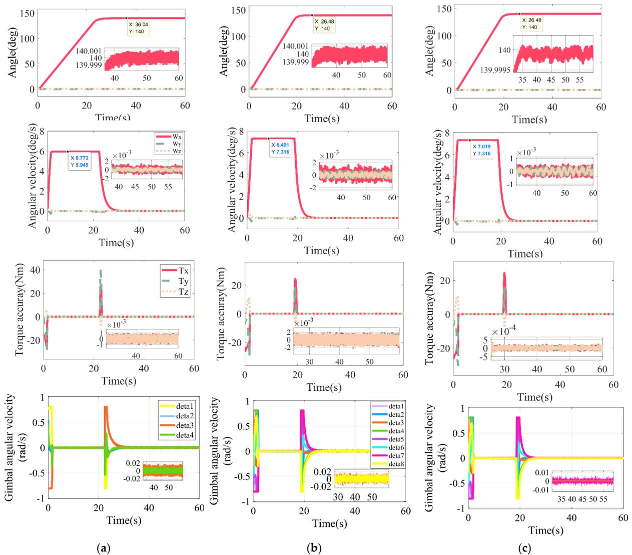
Figure 11. Simulation results of large-angle attitude maneuver. (a) Large 4-SGCMGs, (b) 8-SGCMGs, (c) Reconfiguration of 8-SGCMGs into 4-SGCMGs.
