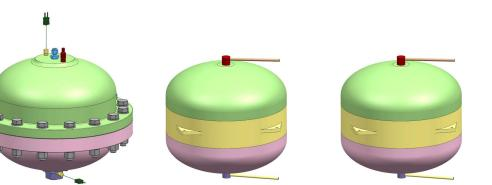
**Figure 7.** Propellant Tank development logic: (**a**) breadboard model, (**b**) qualification model, (**c**) engineering model.
