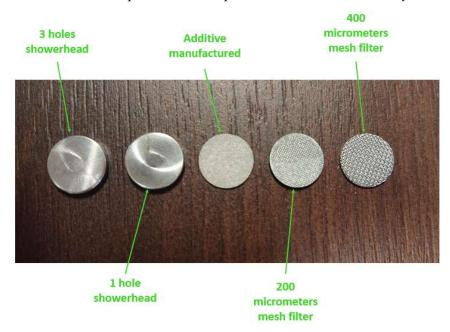
Figure 13. Different injector types.
