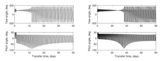
Figure 5. The time histories of thrust direction angles with transfer time of 40 days and 80 days.
