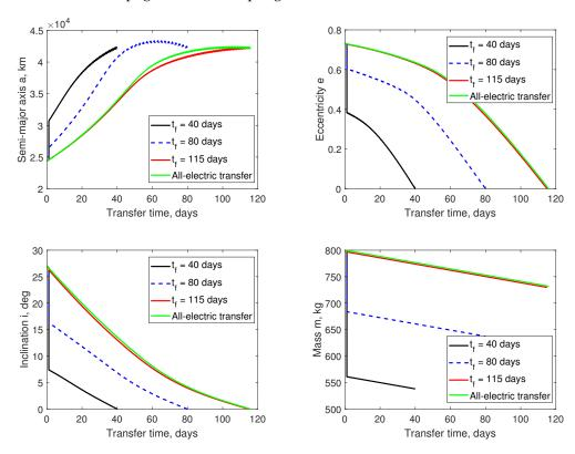
**Figure 4.** The time histories of the semi-major axis, eccentricity, inclination and mass of hybrid transfer orbit with transfer time of 40 days, 80 days, 115 days and all-electric transfer orbit.
