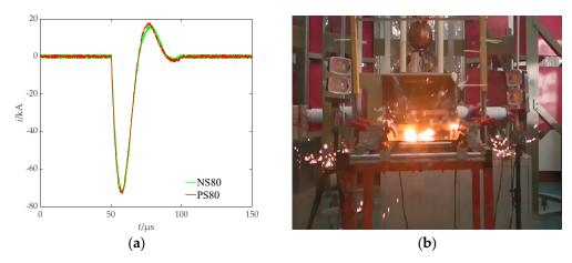
**Figure 7.** Acquisition results of simulated lightning strike test: (**a**) test current waveform; (**b**) simulate lightning test phenomenon.
