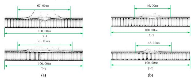
**Figure 9.** Internal damage images by X-ray CT scanning: (**a**) scanning results of the NS80 specimen; (**b**) scanning results of the PS80 specimen.
