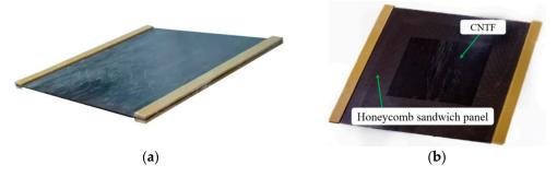
Figure 5. Specimens after curing: (a) unprotected specimen; (b) protected specimen.
