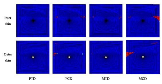
Figure 19. Damage distribution of skin in the PS80 specimen.
