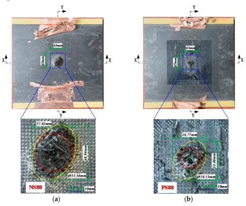
Figure 8. Apparent damage of specimens: (a) NS80 specimen; (b) PS80 specimen.
