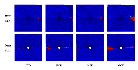
Figure 20. Damage distribution of skin in the NS80 specimen.
