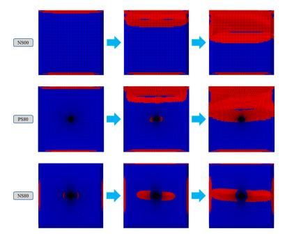
Figure 21. The damage distribution and evolution for honeycomb core in specimens.
