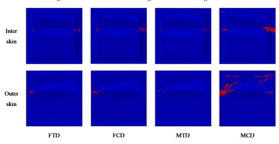
in the middle of the skin of the NS80 specimen is too large, and the stress concentration is significant, which leads to damage before the damage in the chamfer zone occurs.
