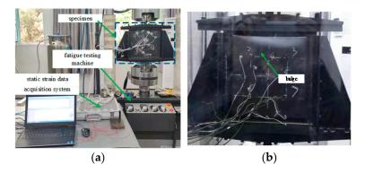
Figure 11. Axial compression test: (a) axial compression test site; (b) specimen failure scenario.
