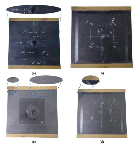
**Figure 14.** Axial compression damage morphology: (**a**) the outer skin side of the NS80 specimen; (**b**) the inner skin side of the NS80 specimen; (**c**) the outer skin side of the PS80 specimen; (**d**) the inner skin side of the PS80 specimen.
