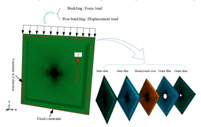
Figure 15. Schematic diagram of finite element model and boundary conditions.
