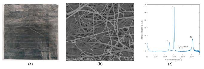
**Figure 2.** CNTF fabricated by FCCVD and its related properties: (**a**) CNTF samples; (**b**) SEM result; (**c**) RS result.
