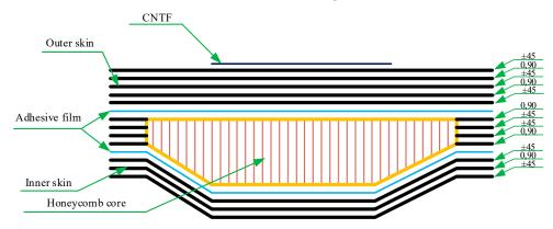
Figure 4. Laying sequence of honeycomb panel specimens (not in scale).
