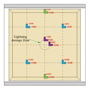
specimen for damage detection in the compression process. The final strain gauge layout of the honeycomb sandwich specimen is shown in Figure 10.
