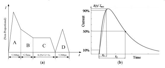
**Figure 6.** Current waveform standard of simulated lightning strike test: (**a**) standard current waveform Data from [32]; (**b**) double exponential pulse waveform.
