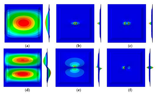
**Figure 16.** Compressive buckling modes of specimens: (**a**) first order buckling mode of the NS00 specimen; (**b**) first order buckling mode of the PS80 specimen; (**c**) first order buckling mode of the NS80 specimen; (**d**) second order buckling mode of the NS00 specimen; (**e**) second order buckling mode of the PS80 specimen; (**f**) second order buckling mode of the NS80 specimen.
