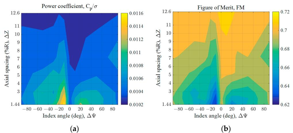
**Figure 18.** Hover performance analyses with respect to various index angles and axial spacings with built-in twist angle =  $-12^\circ$  ( $C_T = 0.0102$ ): (a) Power ( $C_p/\sigma$ ); (b) Figure of Merit (FM).
