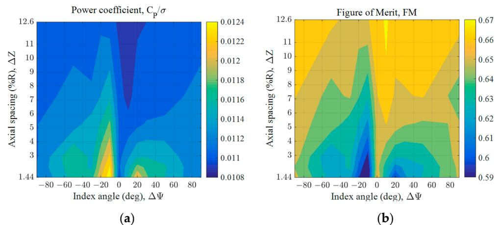
**Figure 13.** Hover performance analyses with respect to various index angles and axial spacings ( $C_T = 0.0102$ ): (a) Power ( $C_P/\sigma$ ); (b) Figure of Merit (FM).
