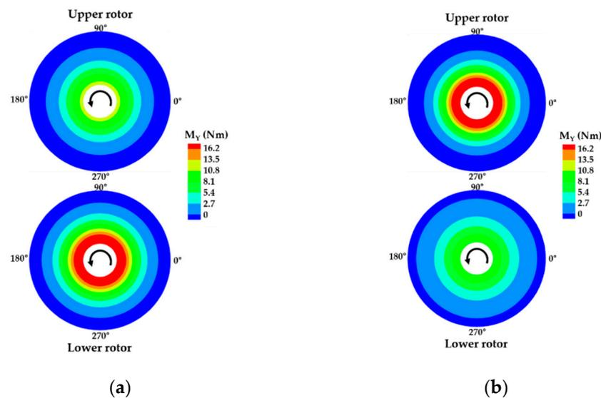
**Figure 15.** Flap bending moment ( $M_Y$ ) distributions at the axial spacing of  $5.27\%R$  ( $C_T = 0.0102$ ): (a) Index angle =  $-10^\circ$ ; (b) index angle =  $10^\circ$ .
