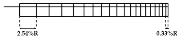
Figure 6. Aerodynamic panels in CAMRAD II model.
