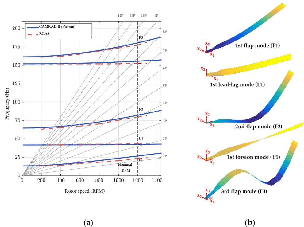
**Figure 8.** Validation for natural frequencies of rotating blade with RCAS [20]: (a) Fan plot; (b) mode shapes at the nonrotating condition.
