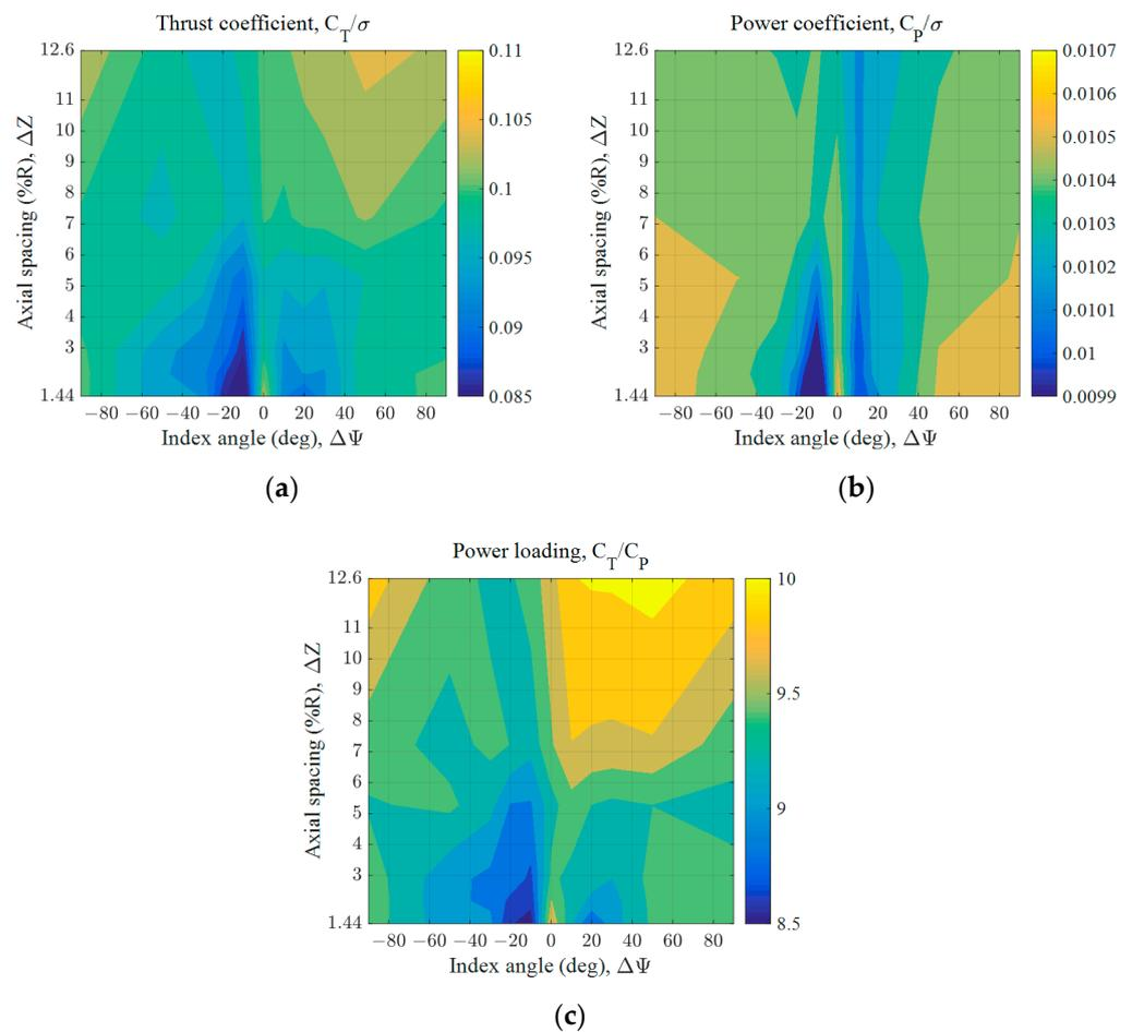
**Figure 10.** Hover performance analyses with respect to various index angles and axial spacings (collective pitch angle =  $12^\circ$ ): (a) Thrust ( $C_T/\sigma$ ); (b) power ( $C_P/\sigma$ ); (c) power loading ( $C_T/C_P$ ).
