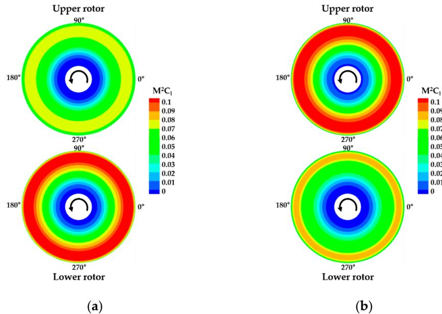
**Figure 16.** Section lift force ( $M^2C_1$ ) distributions at the axial spacing of 5.27%R ( $C_T = 0.0102$ ): (a) Index angle =  $-10^\circ$ ; (b) index angle =  $10^\circ$ .
