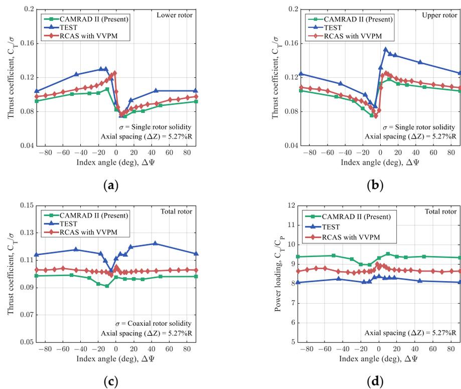
**Figure 9.** Validation for hover performance analyses of coaxial co-rotating rotor in terms of index angle with previous results [21] (collective pitch angle = 12°): (a) Lower rotor thrust ( $C_T/\sigma$ ); (b) upper rotor thrust ( $C_T/\sigma$ ); (c) total rotor thrust ( $C_T/\sigma$ ); (d) total rotor power loading ( $C_T/C_P$ ).
