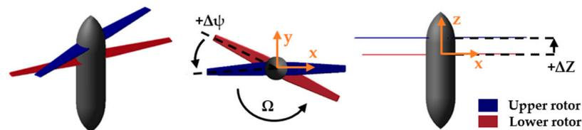
**Figure 3.** Index angle ( $\Delta\Psi$ ) and axial spacing ( $\Delta Z$ ) for coaxial co-rotating rotor.
