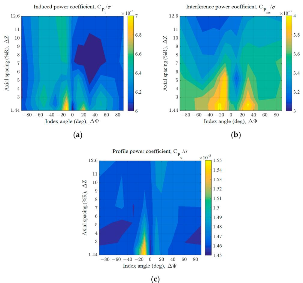
**Figure 14.** Rotor power components with different index angles and axial spacings ( $C_T = 0.0102$ ): (a) Induced power ( $C_{p_i}/\sigma$ ); (b) interference power ( $C_{p_{int}}/\sigma$ ); (c) profile power ( $C_{p_o}/\sigma$ ).
