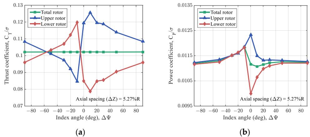
**Figure 12.** Hover performance analyses in terms of index angle ( $C_T = 0.0102$ ): (a) Thrust ( $C_T/\sigma$ ); (b) power ( $C_P/\sigma$ ).
