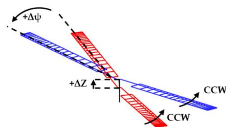
Figure 7. CAMRAD II model for a coaxial co-rotating rotor in hover.
