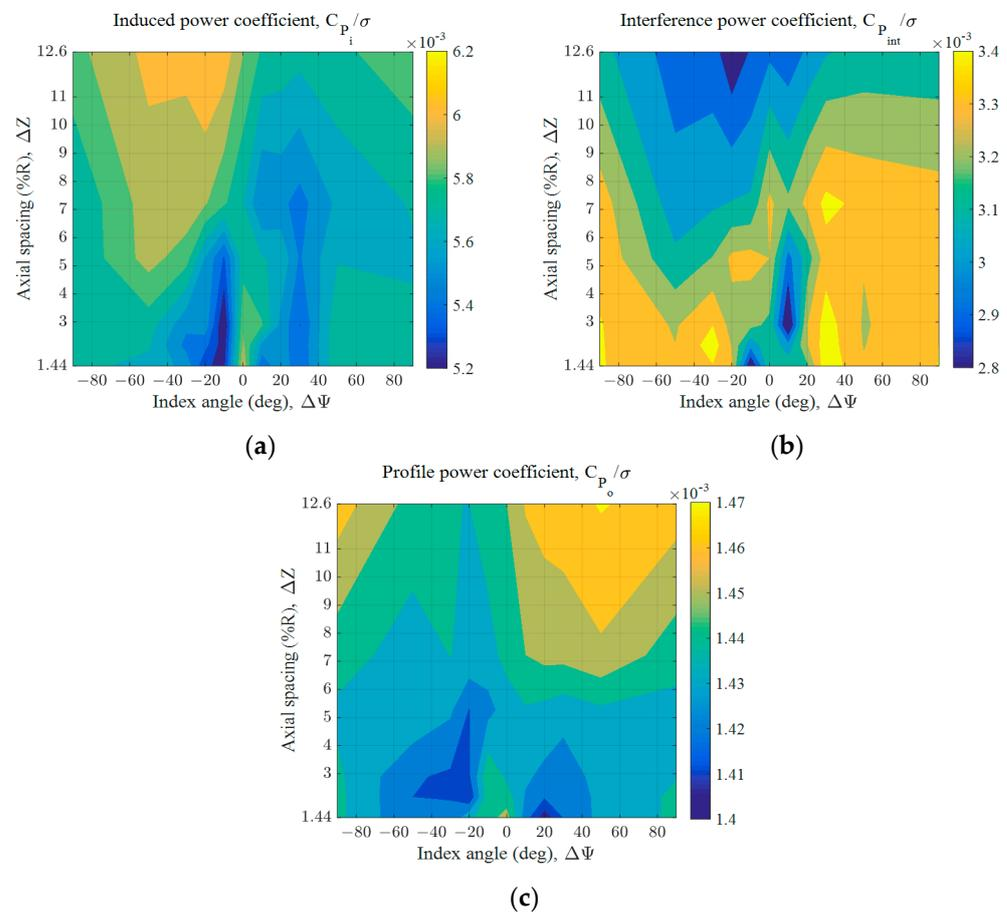
**Figure 11.** Rotor power components with different index angles and axial spacings (collective pitch angle =  $12^\circ$ ): (a) Induced power ( $C_{P_i}/\sigma$ ); (b) interference power ( $C_{P_{int}}/\sigma$ ); (c) profile power ( $C_{P_o}/\sigma$ ).
