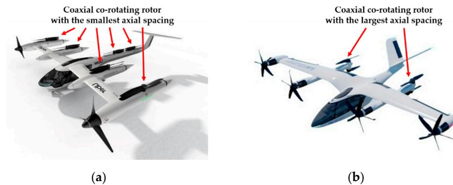
**Figure 2.** Coaxial co-rotating rotors with different axial spacings for eVTOL aircraft: (a) Uber; (b) Korea Aerospace Industries.
