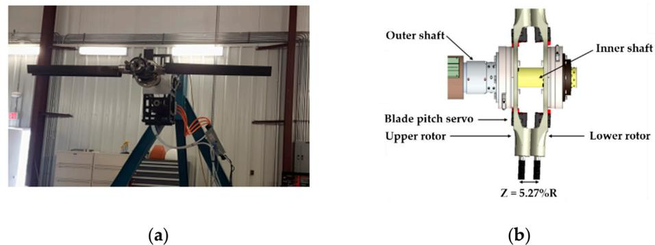
**Figure 4.** Coaxial co-rotating rotor model for test [1,20,21]: (a) Test stand; (b) rotor hub.
