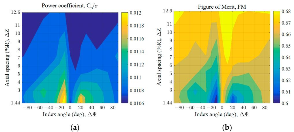
**Figure 17.** Hover performance analyses with respect to various index angles and axial spacings with blade taper ratio = 0.8 ( $C_T = 0.0102$ ): (a) Power ( $C_P/\sigma$ ); (b) Figure of Merit (FM).
