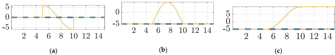
**Figure 3.** Optimal Trajectories from Pontryagin's Method with time in seconds on the abscissas. (a) angular acceleration  $\dot{\omega}(t)$  on the ordinate, (b) angular velocity  $\omega(t)$  on the ordinate, (c) angular displacement  $\theta(t)$  on the ordinate. Note the similarity in the (c) to Figure 2a.
