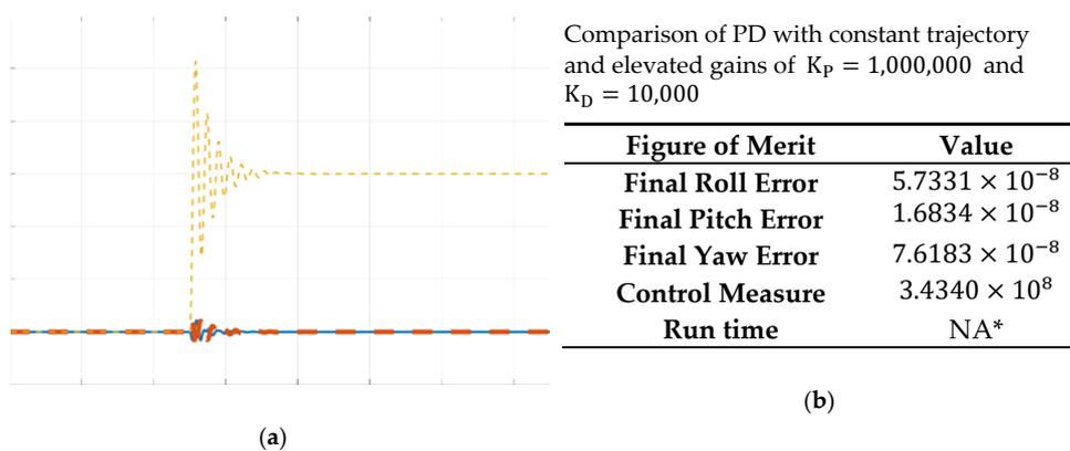
**Figure 4.** System response of PD control with constant trajectory. (a) Plot of Euler angles during the maneuver. Roll is solid blue, pitch is thick dashed red, yaw is thin dashed yellow (b) Characteristics of the response. \* Note, this run time was found to be much lower due to differences in available processing power and when compared to re-simulations of some of the above methods, found to be comparable.
