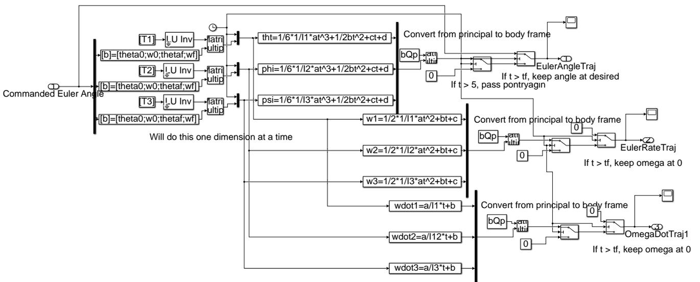
Figure A4. Pontryagin based Trajectory Generation.
