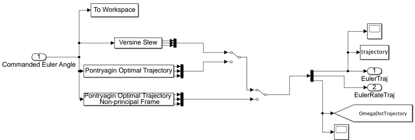
Figure A2. Trajectory generation block model.
