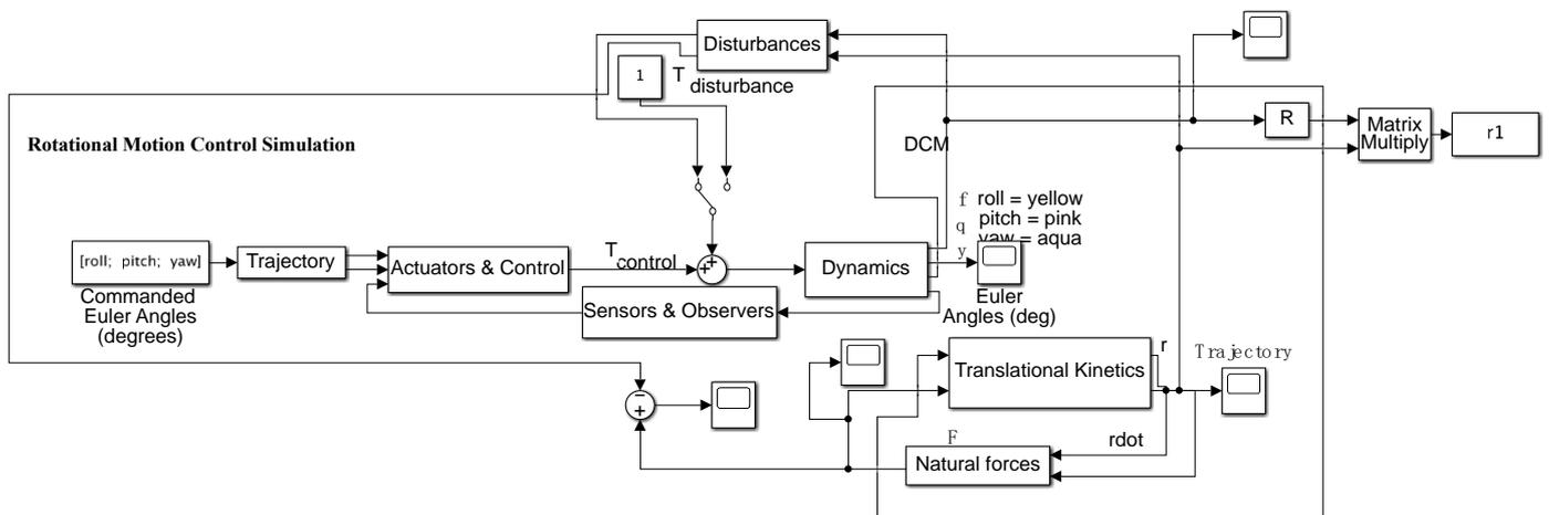
**Figure A1.** Simulink Model Complete display of all SIMULINK systems and subsystems.
