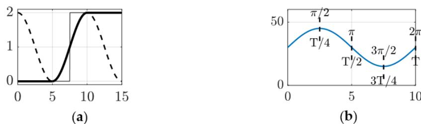
**Figure 2.** (a) Piecewise sinusoidal trajectory with a slew time/maneuver time of 5 s and a quiescent time of 5 s before and after the slew (b) A nominal sine wave used to reveal relationship between points on the curve’s time and phase angle.
