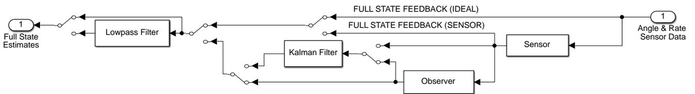
Figure A6. Sensors and Observers block model.
