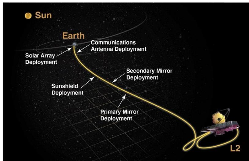
**Figure 1.** James Webb telescope positions in the second Lagrange point, L2 from which attitude maneuvers point the telescope towards distant targets in outer space. [1] Image used consistent with NASA policy, “NASA content (images, videos, audio, etc.) are generally not copyrighted and may be used for educational or informational purposes without needing explicit permissions” [2].
