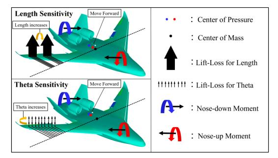
Figure 20. Arms of force of lift-loss in the sensitivity analysis.
