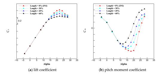
Figure 18. Aerodynamic coefficient of the sensitivity analysis of Length.
