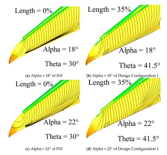
Figure 21. Upper surface limiting streamlines of INI and Design Configuration 1.
