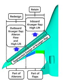
Figure 12. Plan of segmented design of Krueger flap.
