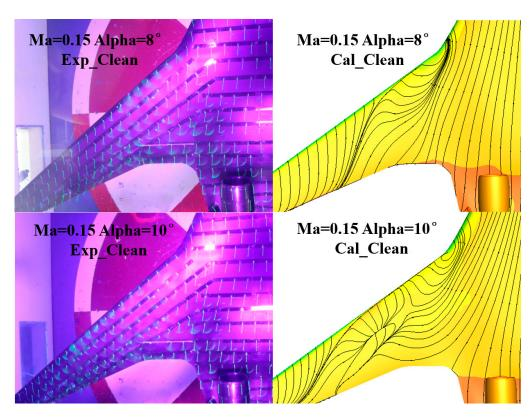
Figure 7. The surface flow of computation and experiment for the clean configuration.
