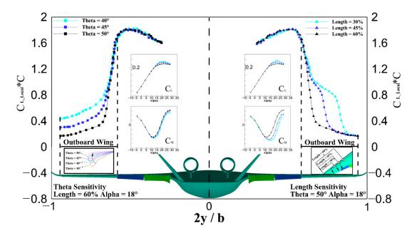
Figure 19. Spanwise lift distribution of the sensitivity analysis.
