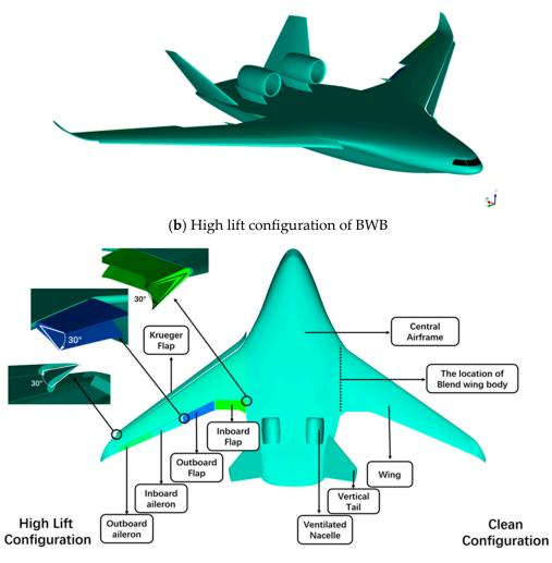
(c) Key parts of configurations of BWB.
