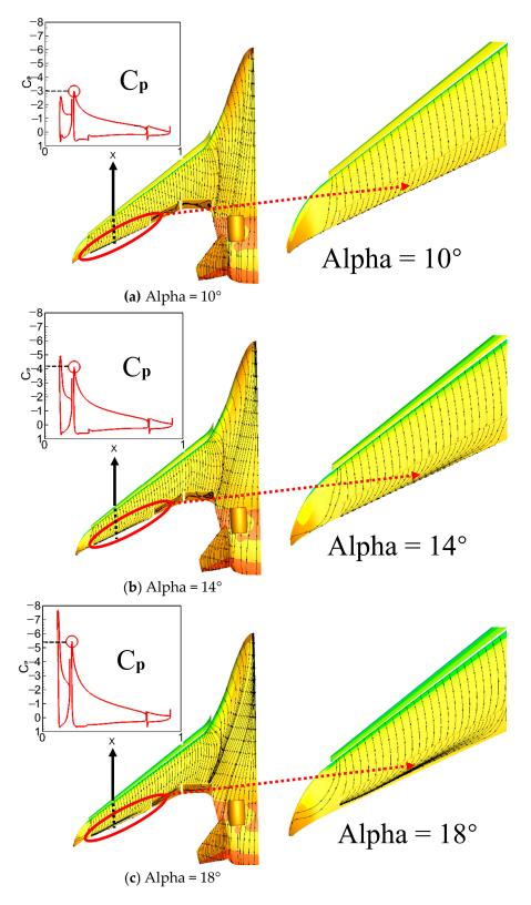
Figure 10. Upper surface limiting streamlines, the local pressure distribution of the high lift configuration.
