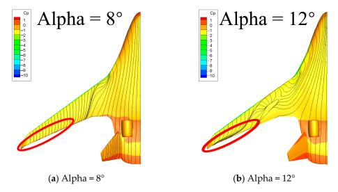
Figure 11. Upper surface limiting streamlines of the clean configuration.
