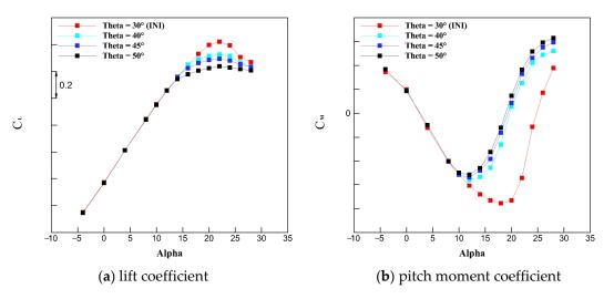
Figure 15. Aerodynamic coefficient of the sensitivity analysis of Theta.
