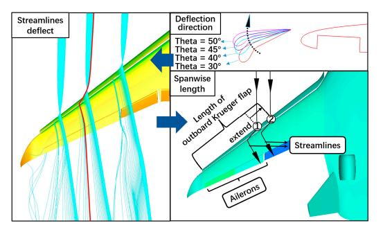
Figure 13. Sensitivity analysis parameter definition and initialization.
