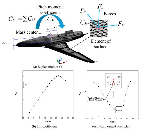
Figure 9. Aerodynamic coefficient of the high lift configuration in real condition.
