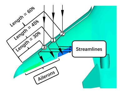
Figure 16. Parameterization of the length of the outboard Krueger flap for sensitivity analysis.
