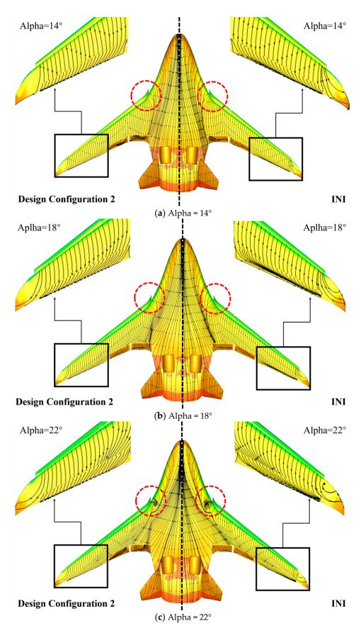
Figure 24. Surface limiting streamlines of INI and Design Configuration 2.
