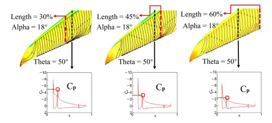
**Figure 17.** Upper surface limiting streamlines; the local pressure distribution of the sensitivity analysis of length.
