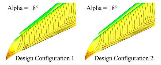
Figure 26. Surface limiting streamlines of Design Configuration 1 and Design Configuration 2.
