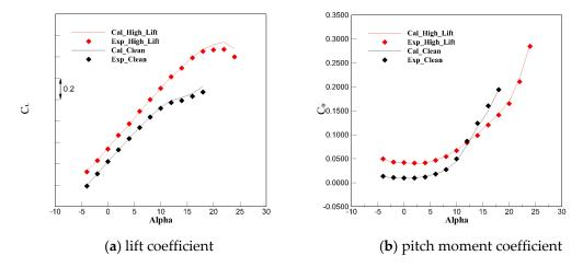
**Figure 6.** Aerodynamic coefficient results of computation and experiment for the clean configuration and the high lift configuration.
