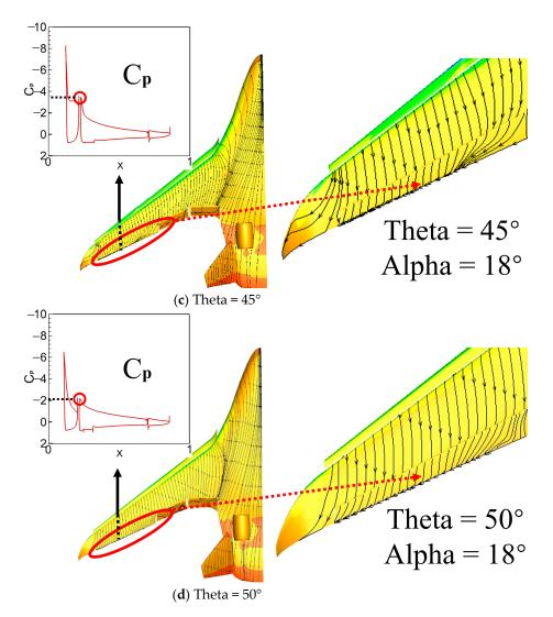
**Figure 14.** Upper surface limiting streamlines, the local pressure distribution of the sensitivity analysis of Theta.
