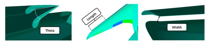
**Figure 27.** Adjustment parameters of the Krueger flap for the improvement of aileron surface flow state.
