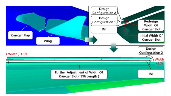
Figure 23. Redesign of the width of the outboard Krueger flap slot.
