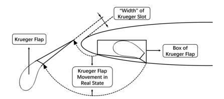
Figure 2. Krueger flap movement in real state.
