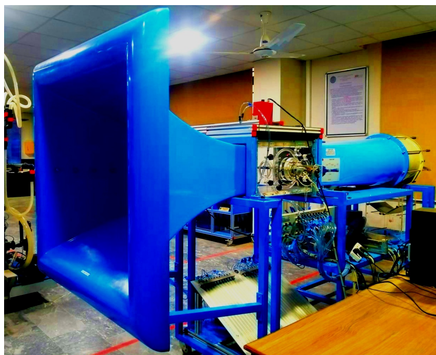
Figure 4. Wind tunnel used in experimental investigation of bullet heads.
