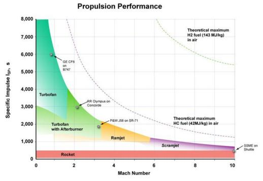
Figure 1. Specific impulse of different engines [1].
