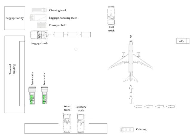
Figure 1. Deployment of ground handling equipment before changes were applied.
