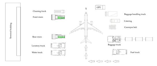
Figure 2. Deployment of ground handling equipment after changes were applied.
