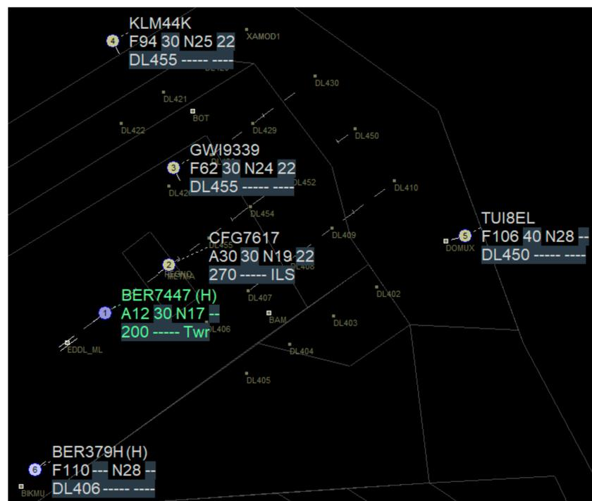
**Figure 1.** Aircraft radar labels next to aircraft circle icons (containing sequence numbers) flying within Düsseldorf approach airspace shown on DLR's radar display RadarVision [93]. The five shaded label cells in the second and third label lines may depict the last ATCo command value for a certain command type (altitude, speed, direction, rate of altitude change, miscellaneous).
