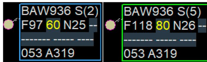
**Figure 3.** Solution aircraft radar labels with yellow ABSR output expecting attention-based ATCo confirmation and colored label frames in different states; left: light blue frame in saliency level “2” as visual check gaze for ABSR output is pending, right: green frame in saliency level “5” as visual check gaze has confirmed and time for potential manual ASBR output correction is running.
