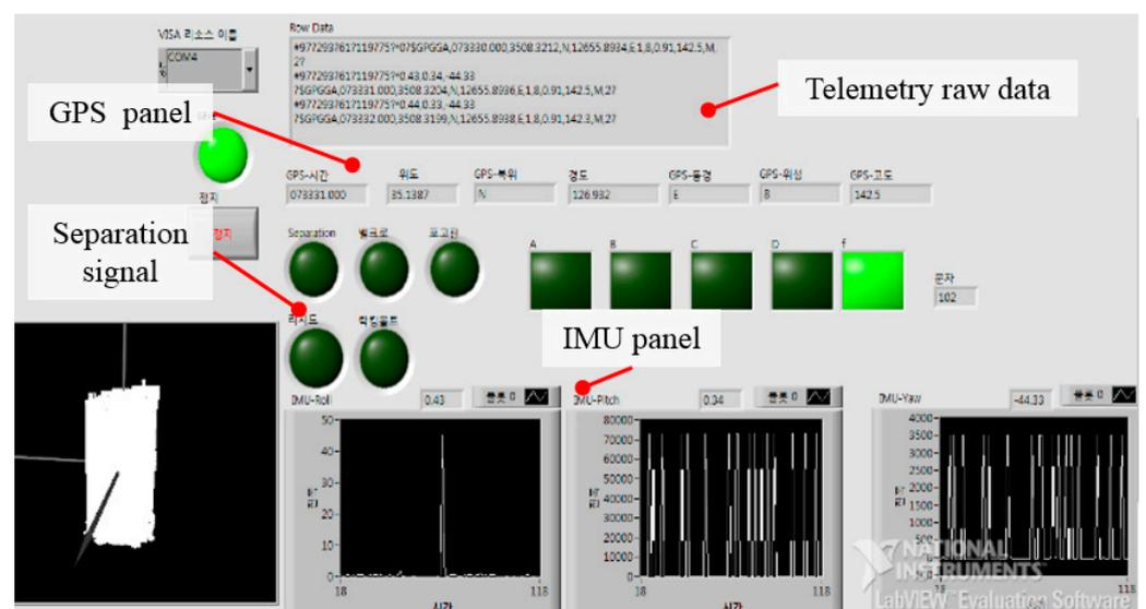
Figure 9. Captured monitor view of the software developed for the DHRM CanSat ground station.
