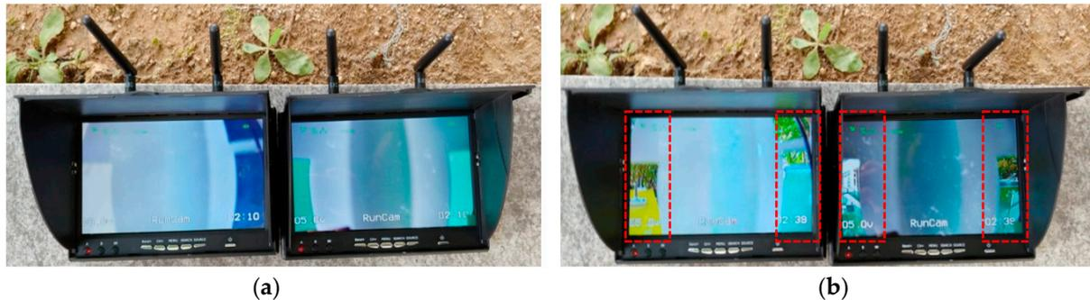
Figure 12. Images captured by the onboard cameras of the CanSat (a) before and (b) after deployment of the solar panels.
