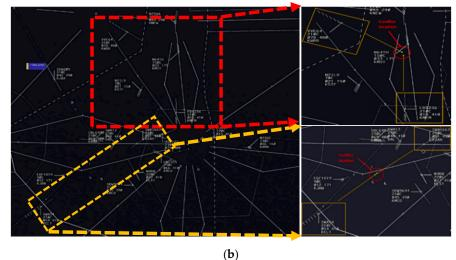
**Figure 2.** Example scenarios: (a) Layout of aircraft during an experiment using one of the scenarios; (b) Example of aircraft conflicts highlighted in red and yellow (left side shows the aircraft layout at a certain point in time, and the right side shows the future conflict locations.
