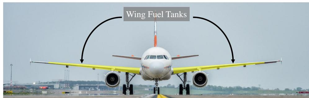
**Figure 1.** The fuel tank chambers of an aircraft are mainly situated in the wings, but also within the center of the fuselage.
