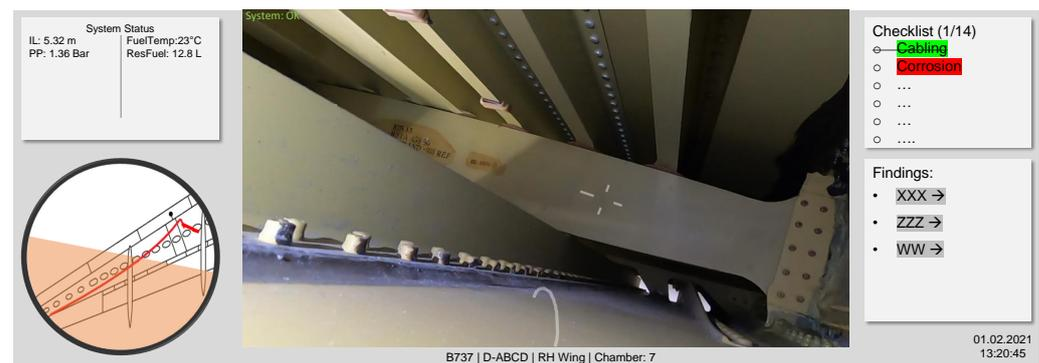
**Figure 17.** The prototype for the human machine interface for controlling the endoscopic system and performing the general visual inspection is demonstrated using an empty fuel tank.
