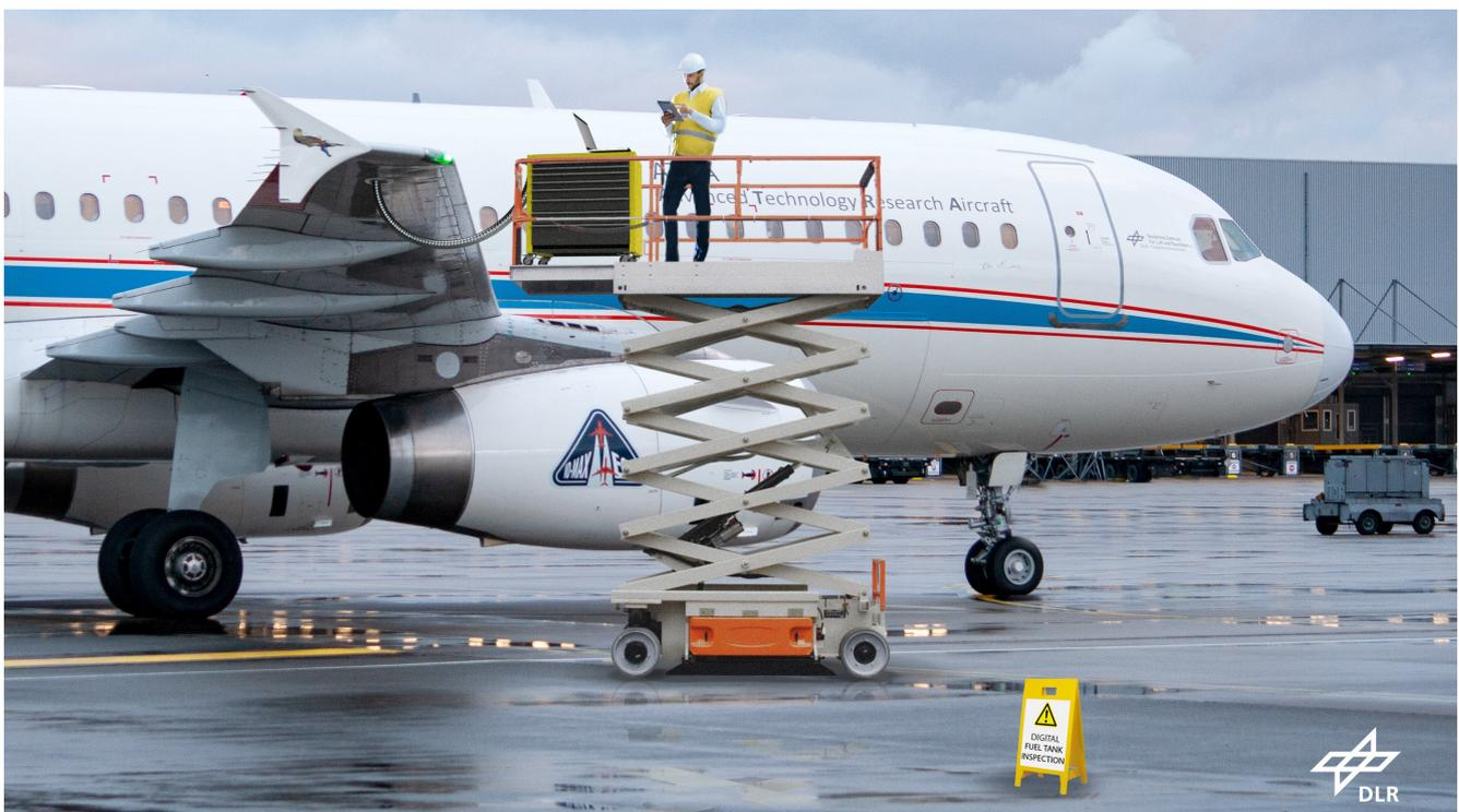
**Figure 11.** Conceptual visualization of a future fuel tank maintenance process. Therefore, a hose-like structure can be attached to the wing fuel tank from a working platform to insert an endoscopic probe.
