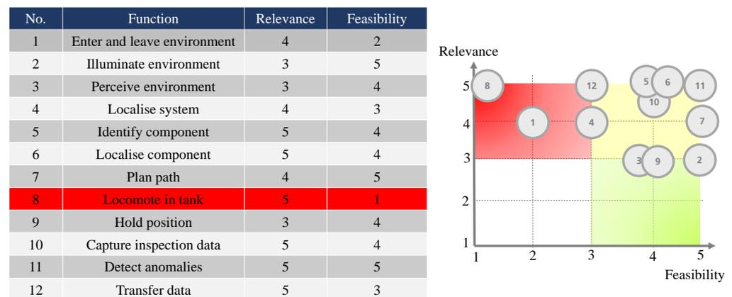
**Figure 8.** Definition and Assessment of Abstract Basic Functions for Tank Inspection Process.
