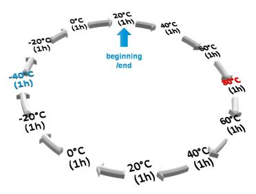
**Figure 18.** Thermal cycling performed on a 10 cm  $\times$  10 cm TiO<sub>2</sub>–SiO<sub>2</sub> grid architecture divided into three steps: a first increase from 20 °C to 80 °C followed by a decrease down to -40 °C, while the last increase is performed to reach 20 °C. Each temperature level lasts 1 h.
