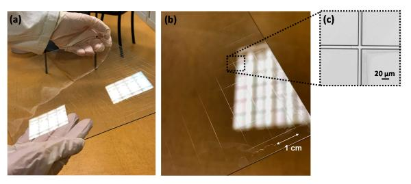
**Figure 9.**  $\text{TiO}_2\text{-SiO}_2$  grid architecture on a large substrate composed of 62 guides. (a) Overview of the sensor, (b) corresponding zoom showing the 1 cm separation between two consecutive lines and (c) microscope image of the doubled exposed zone.
