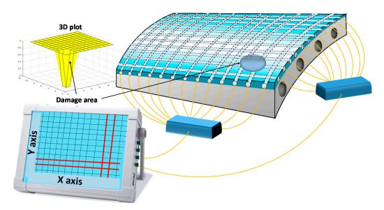
**Figure 1.** Final architecture of the 2D sol–gel matrix sensor for damage detection. The sensor is based on a grid of optical waveguides. An impact on the plane leads to the degradation or the rupture of one or more waveguides. Thanks to the particular 2D structure of the sensing material, the identification of the impacted damage allows the damage localization.
