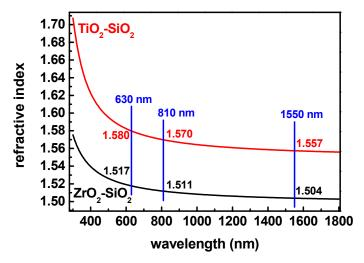
**Figure 11.** Refractive index of  $TiO_2$ – $SiO_2$  (red line) and  $ZrO_2$ – $SiO_2$  (black line) obtained by the ellipsometry technique. The layers were insolated by UV photons and thermally treated.
