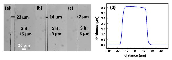
**Figure 4.**  $\text{TiO}_2\text{-SiO}_2$  patterns obtained using the amplitude mask with different slits at 15  $\mu$ m, 8  $\mu$ m and 3  $\mu$ m. Microscope observations (reflection x20) of (a) line obtained with a slit of 15  $\mu$ m in width, (b) line obtained with a slit of 8  $\mu$ m and (c) line obtained with a slit of 3  $\mu$ m. (d) Profilometer measurement of (a).
