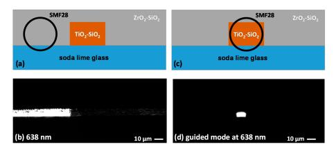
**Figure 15.** Injection of visible light (638 nm) in the architecture composed of the  $TiO_2$ – $SiO_2$  core deposited on soda-lime glass and surrounded by the  $ZrO_2$ – $SiO_2$  cladding. (a) Diagram of the SMF28 misaligned with the core, (b) corresponding output, (c) diagram of SMF28 aligned with the core and (d) corresponding guided mode. The SMF28 is schematized by black circles.
