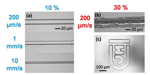
**Figure 7.** Structures obtained by the direct writing technique showing (a) lines obtained at 10% and for different scanning speed (200  $\mu$ m/s, 1 and 10 mm/s), (b) calcinated trace induced at 30% and 200  $\mu$ m/s and (c) Jean Monnet University logo with a 420  $\mu$ m size in height.
