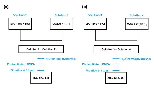
**Figure 2.** Preparation of the different organic–inorganic sol–gel solutions. Material synthesis of (a)  $TiO_2$ – $SiO_2$  and (b)  $ZrO_2$ – $SiO_2$  sols. In both cases, a photoinitiator (DMPA) is added to induce the start of UV-polymerization reactions.
