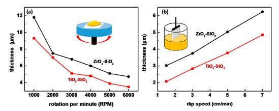
**Figure 5.** Investigation of  $TiO_2$ – $SiO_2$  (red squared curve) and  $ZrO_2$ – $SiO_2$  (black dotted curve) thicknesses using the spin coating (**a**) and the dip coating (**b**) methods.
