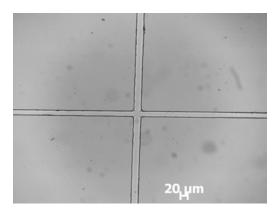
**Figure 6.**  $\text{TiO}_2\text{-SiO}_2$  grid observed using an optical microscope in a reflection mode (×20). The crossed  $\text{TiO}_2\text{-SiO}_2$  area is not affected by the double exposure (360 J/cm<sup>2</sup>).
