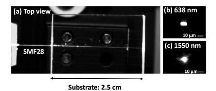
**Figure 14.** Characterization of  $TiO_2$ – $SiO_2$  waveguides (surrounded by air). The figure illustrates: (a) top-view of the waveguide injection at 638 nm, (b) output optical guided mode at 638 nm and (c) guided mode at 1550 nm.
