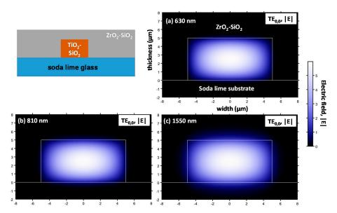
**Figure 13.** Simulated  $TE_{00}$  mode of a  $TiO_2$ – $SiO_2$  waveguide deposited on soda-lime glass and surrounded by the  $ZrO_2$ – $SiO_2$  cladding and operating at (a) 630 nm, (b) 810 nm and (c) 1550 nm. The thicknesses and widths are 5  $\mu$ m and 10  $\mu$ m, respectively.
