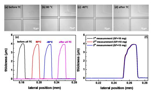
Figure 19. Thermal cycling (TC) effect on a  $\text{TiO}_2$ – $\text{SiO}_2$  grid architecture. Microscope images of the grid area are given (a) before the thermal cycling, (b) after being thermally treated at 80 °C, (c) -40 °C and (d) after all the consecutive thermal treatments. (e) Corresponding profilometer measurements (SF = 10 mg) and (f) profilometer measurements of the structure submitted to the full thermal cycling with SF of 10 mg (black and red lines) and 15 mg (blue line).
