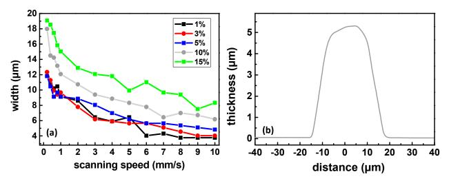
**Figure 8.** Characterization of the photo-induced patterns using the Dilase 750 facility. (a) Width of the structures as a function of the scanning speed for powers ranging from 1% and 15% and (b) profile obtained for a line written at 10% and  $200 \mu m/s$ .
