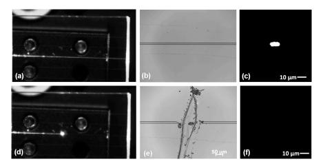
**Figure 16.** Damage detection with a TiO<sub>2</sub>–SiO<sub>2</sub> waveguide operating at 638 nm showing: (a) top-view of the unaffected guide before the impact, (b) corresponding microscope image and (c) guided mode. After the impact: (d) top-view, (e) microscope image and (f) absence mode observation.
