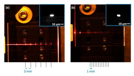
**Figure 17.** Top-view of  $TiO_2$ – $SiO_2$  waveguide grid after signal injection at 638 nm for (a) 6 perpendicular waveguides spaced by 3 mm and (b) 12 perpendicular waveguides spaced by 1 mm. In both cases, the corresponding inset illustrates the guided mode at 638 nm, and the waveguides are surrounded by air.
