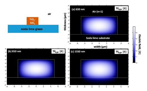
Figure 12. Simulated transverse electric  $TE_{00}$  mode of a  $TiO_2$ – $SiO_2$  waveguide deposited on a sodalime glass surrounded by air and operating at (a) 630 nm, (b) 810 nm and (c) 1550 nm. The thicknesses and widths are 5  $\mu$ m and 10  $\mu$ m, respectively.
