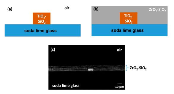
Figure 10. Two configurations of the photonic device deposited on soda-lime glass. (a)  $TiO_2-SiO_2$  core without cladding and surrounded by air. (b)  $TiO_2-SiO_2$  core buried in a  $ZrO_2-SiO_2$  coating and (c) output light of the  $TiO_2-SiO_2$  core waveguide with  $ZrO_2-SiO_2$  cladding obtained experimentally.
