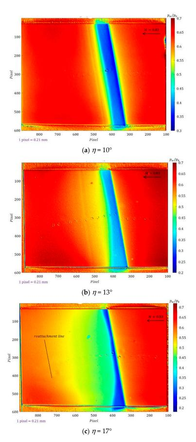
**Figure 5.** Global surface pressure distribution for M=0.83 and  $\lambda=10^\circ$ : (a)  $\eta=10^\circ$ ; (b)  $\eta=13^\circ$ ; (c)  $\eta=17^\circ$ .
