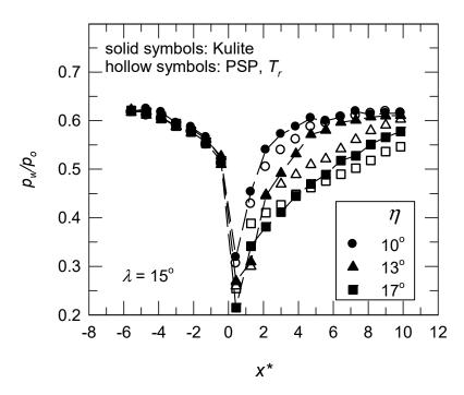
**Figure 8.** Longitudinal pressure distribution at the centerline for M = 0.83 with a constant offset and recovery factor.
