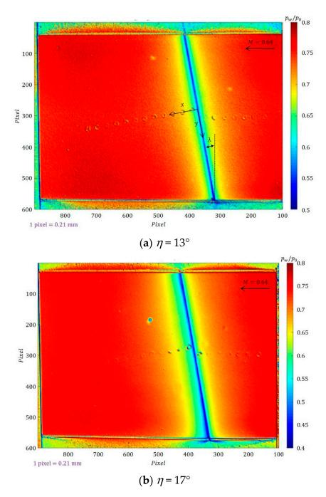
**Figure 4.** Global surface pressure distribution for Mach number (M) = 0.64 and swept angle ( $\lambda$ ) =  $10^{\circ}$ : (a) convex-corner angle ( $\eta$ ) =  $13^{\circ}$ ; (b)  $\eta$  =  $17^{\circ}$ .
