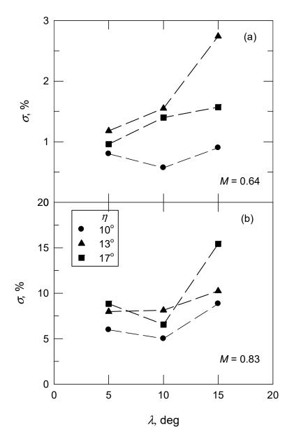
**Figure 11.** The difference between longitudinal pressure distributions using pressure-sensitive paint (PSP) and Kulite sensors: (a) M = 0.64; (b) M = 0.83.
