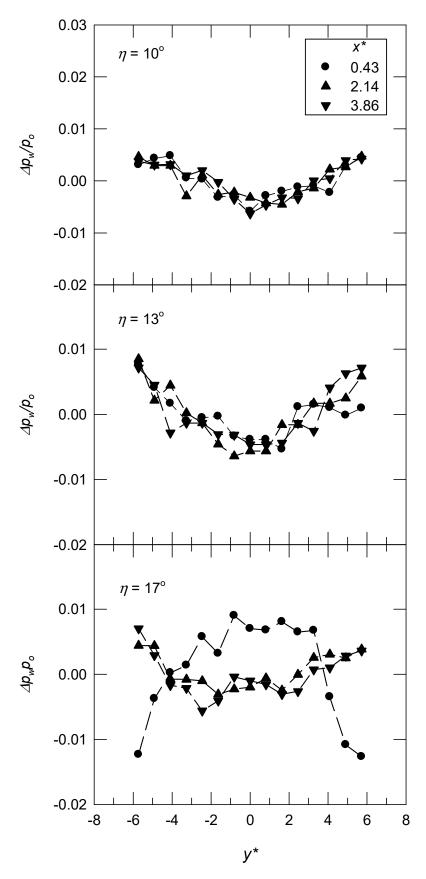
**Figure 9.** Spanwise pressure distribution for M = 0.64 and  $\lambda = 10^{\circ}$ .
