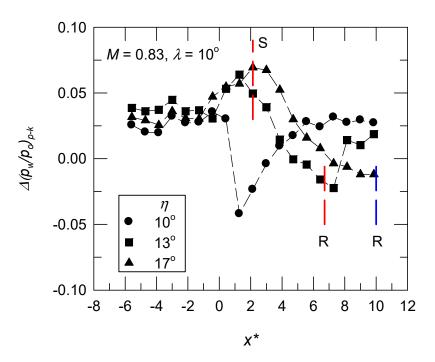
**Figure 13.** Local flow structure of the difference between PSP and Kulite sensors for M = 0.83 and  $\lambda = 10^{\circ}$ .
