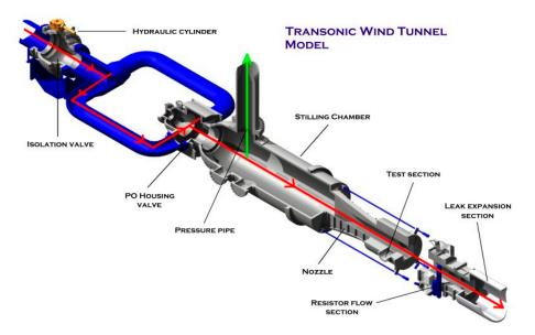
**Figure 1.** Aerospace Science and Technology Research Center, National Cheng Kung University (ASTRC/NCKU) transonic wind tunnel.
