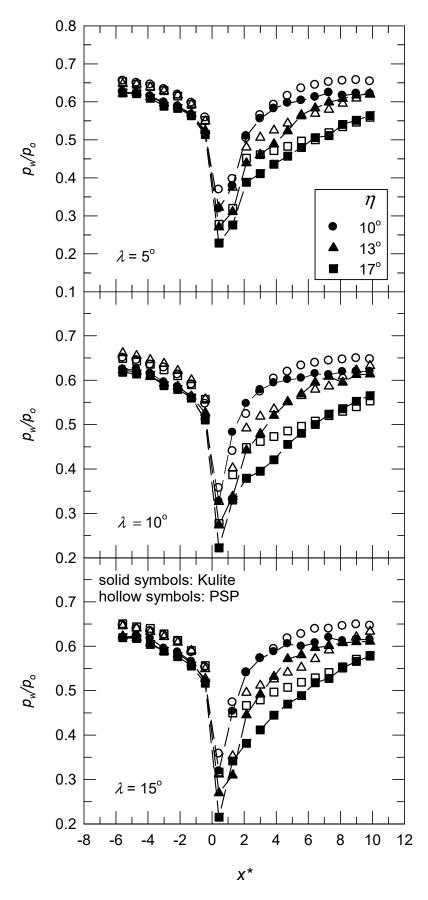
**Figure 7.** Longitudinal pressure distribution at the centerline for M = 0.83.
