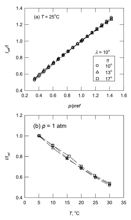
**Figure 3.** Calibration curves for Pt (II) meso-Tetra (pentafluorophenyl) porphine (PtTFPP): (a) temperature (T) = 25 °C; (b) pressure (p) = 1 atm.
