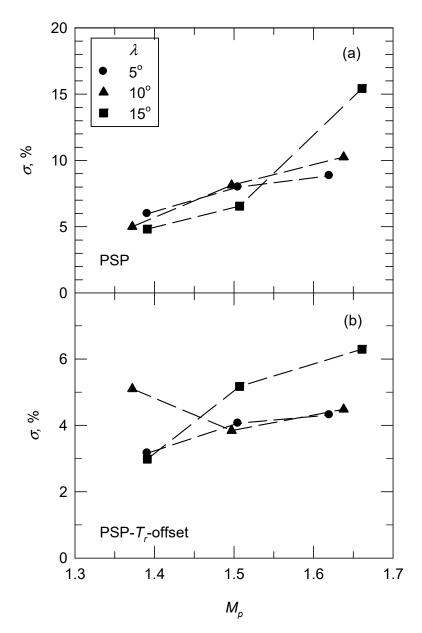
**Figure 12.** The difference between longitudinal pressure distributions using PSP and Kulite sensors, corrected by a reference pressure tap and a recovery factor: (a) No temperature correction; (b) Temperature correction with a constant recover factor.
