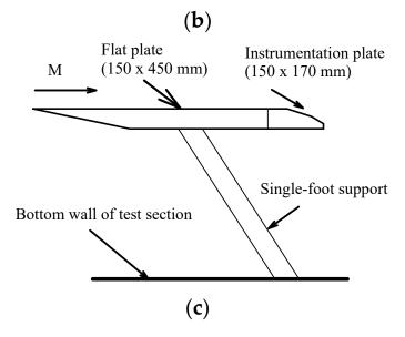
**Figure 2. Swept convex corner.** (a) top view for swept convex corner; (b) side view for swept convex corner; (c) model support.
