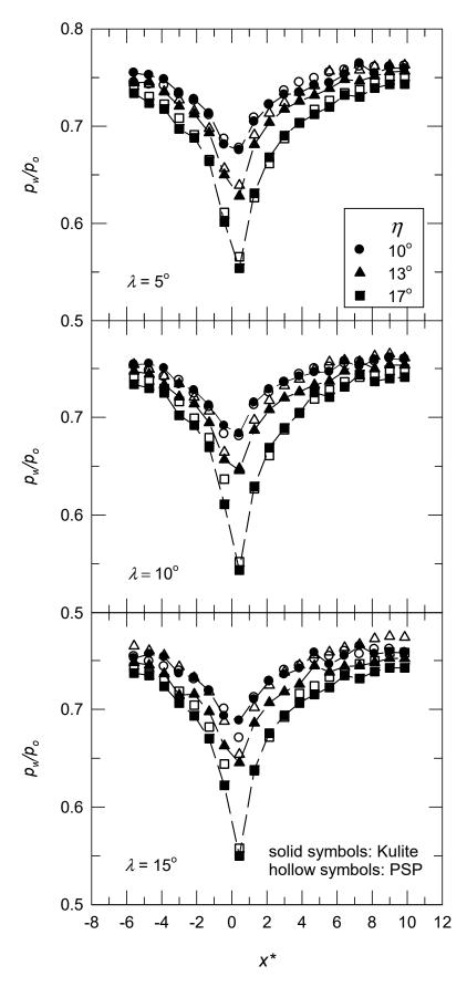
**Figure 6.** Longitudinal pressure distribution at the centerline for M = 0.64.
