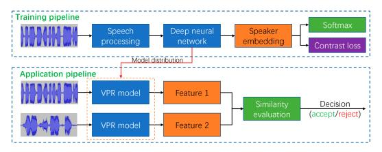
Figure 7. The voiceprint recognition (VPR) pipelines.
