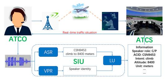
**Figure 1.** The air traffic control (ATC) procedure and spoken instruction understanding (SIU) roles in ATC.
