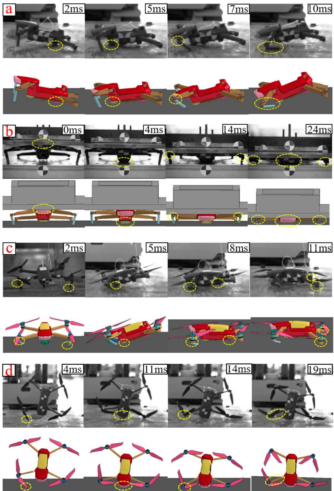
**Figure 6.** Comparison of deformation response of full-size model. (a) Drop test of drone components. (b) Drop-weight test of drone components. (c) Drop test of drone positive posture. (d) Drop test of drone vertical posture.
