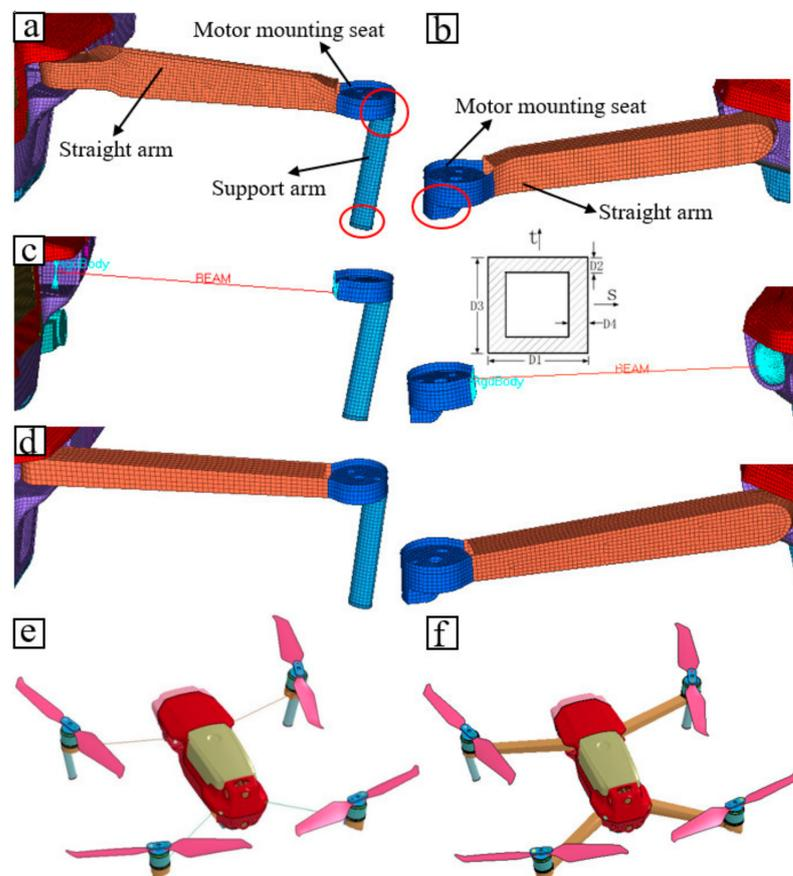
**Figure 12.** (a) Full-size model of front arm. (b) Full-size model of rear arm. (c) Simplified model-5 arm model. (d) Simplified model-6 arm model. (e) Simplified model-5. (f) Simplified model-6.
