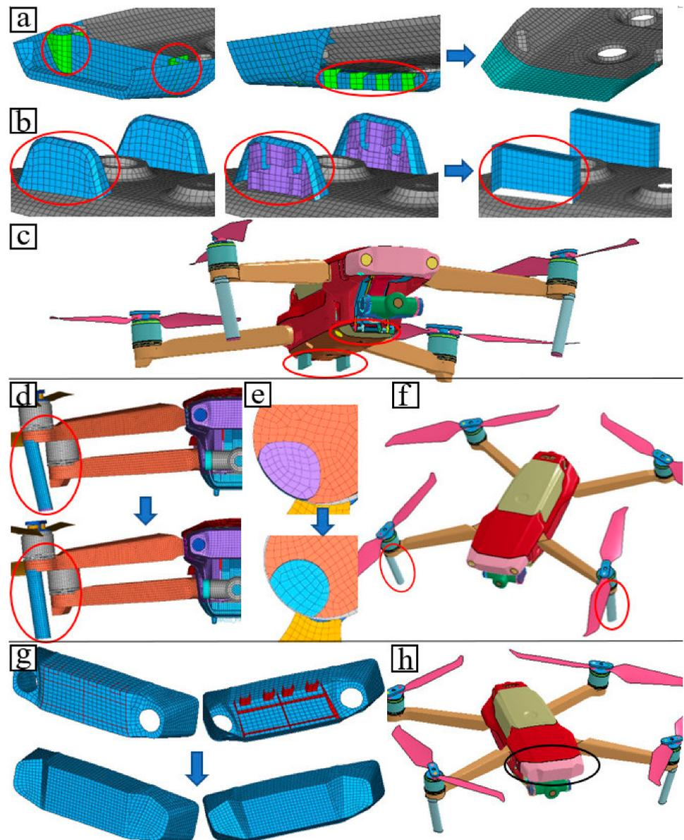
**Figure 14.** (a) Preventer plate. (b) Pedestal (c) Simplified model-8. (d) Elevation view of support arm. (e) Section view of support arm. (f) Simplified model-9. (g) Front shroud. (h) Simplified model-10.
