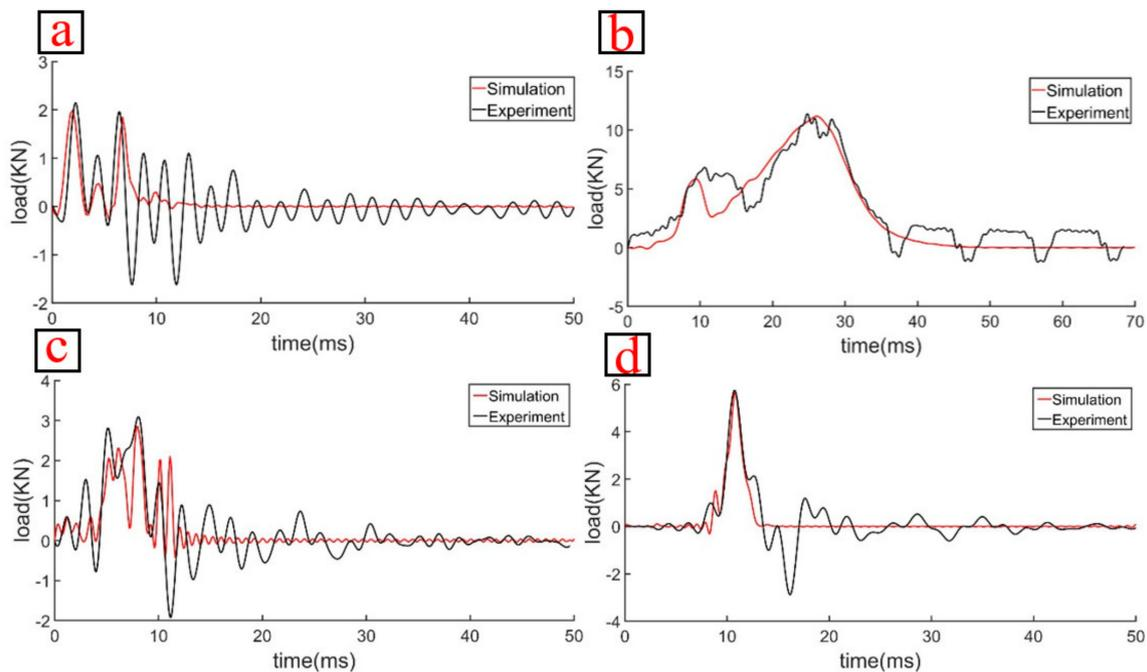
**Figure 7.** Comparison of impact load between simulation and experiment. (a) Drop test of drone components. (b) Drop-weight test of drone components. (c) Drop test of drone positive posture. (d) Drop test of drone vertical posture.
