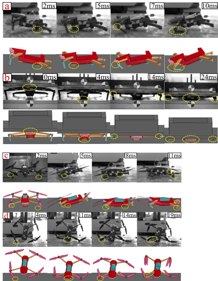
**Figure 18.** Comparison of deformation response of combined simplified model. (a) Drop test of drone components. (b) Drop-weight test of drone components. (c) Drop test of drone positive posture. (d) Drop test of drone vertical posture.
