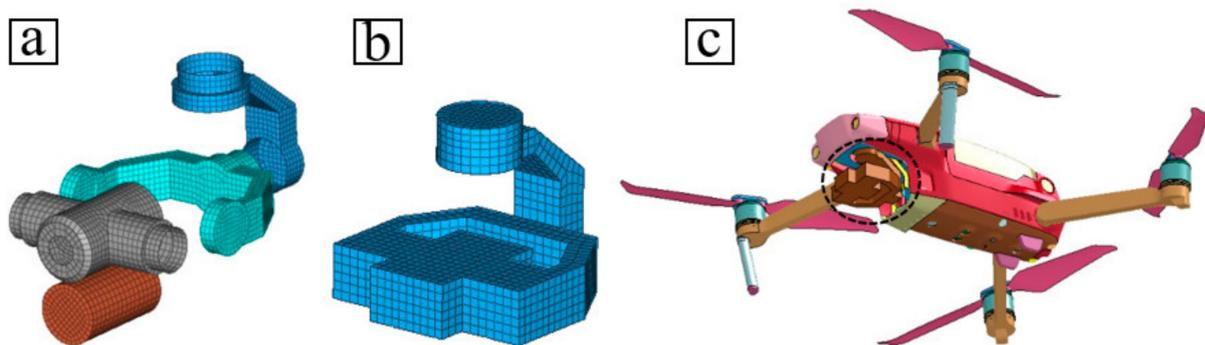
**Figure 10.** (a) Camera full-size model. (b) Camera simplified model. (c) Simplified model-3.
