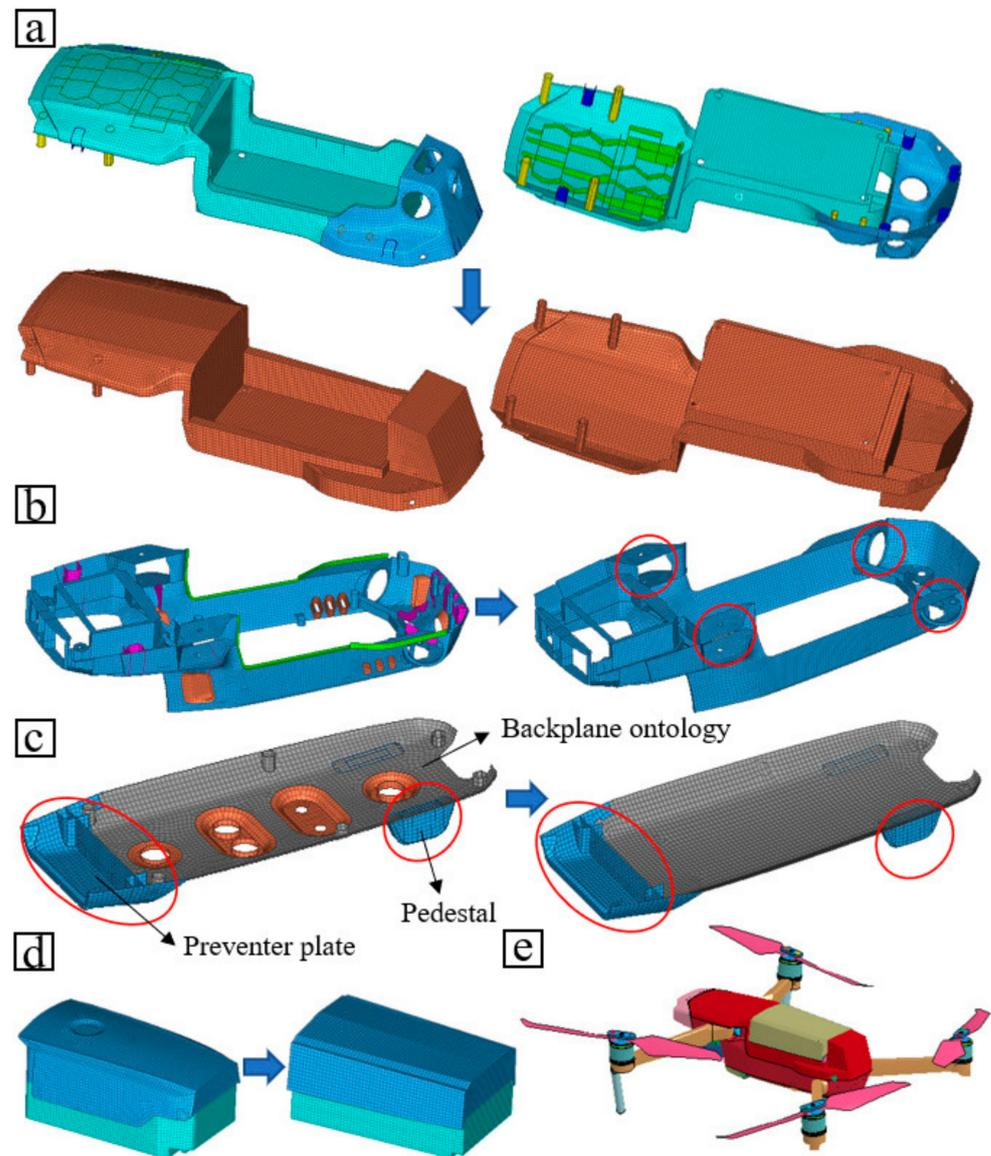
**Figure 13.** (a) Comparison of full-size model and simplified model of upper fuselage. (b) Comparison of full-size model and simplified model of lower fuselage. (c) Comparison of full-size model and simplified model of baseplate (d) Comparison of full-size model and simplified model of battery case (e) Simplified model-7.
