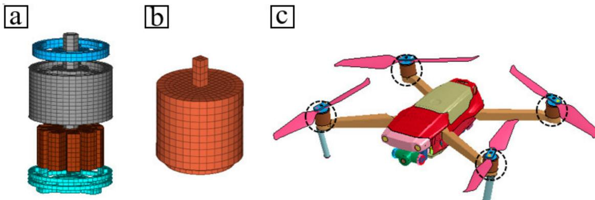
**Figure 9.** (a) Motor full-size model. (b) Motor simplified model. (c) Simplified model-2.
