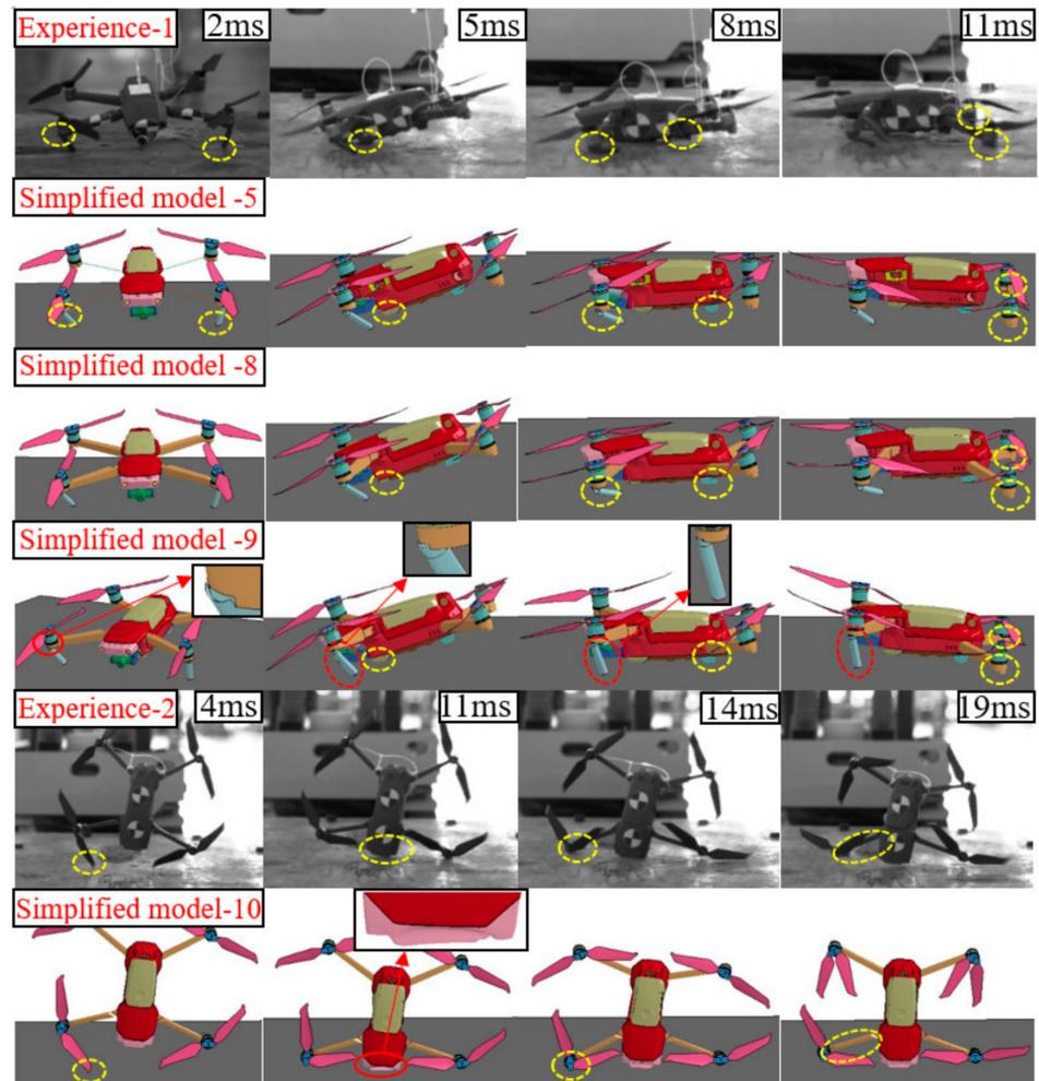
**Figure 16.** Comparison of deformation response of some simplified models.
