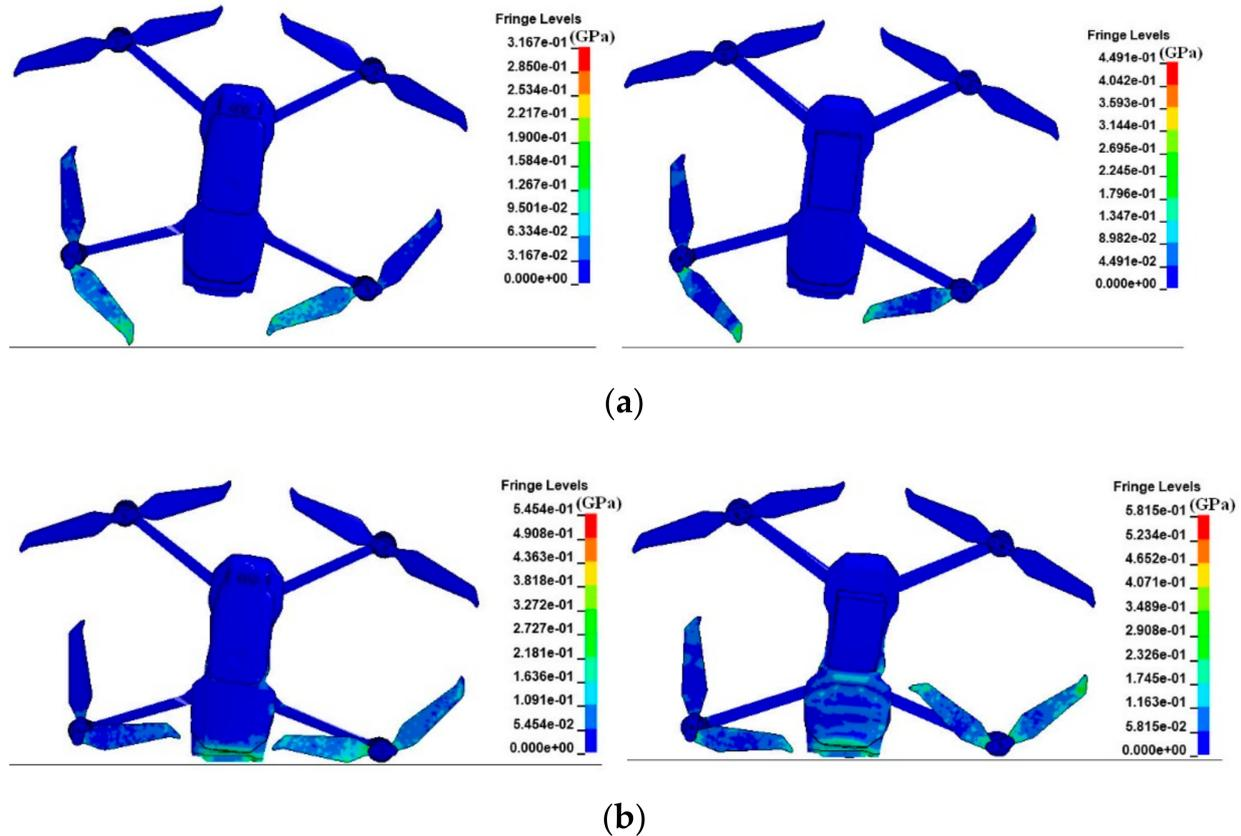
**Figure 21.** Comparison of stress distribution between the simplified model and the full-scale model at the typical time of the complete machine vertical posture drop test. (a)  $4 \times 10^{-3}$  s time. (b)  $11 \times 10^{-3}$  s time.
