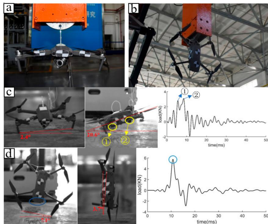
**Figure 5.** (a) Drone positive posture. (b) Drone vertical posture. (c) Drop test results of drone positive posture. (d) Drop test results of drone vertical posture.
