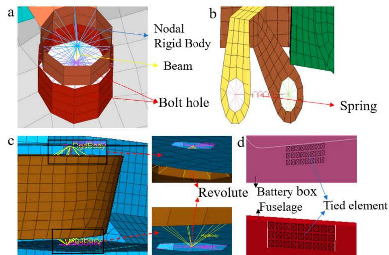
**Figure 2.** (a) Bolted connection. (b) Spring connection. (c) Revolute. (d) Tie-Break.
