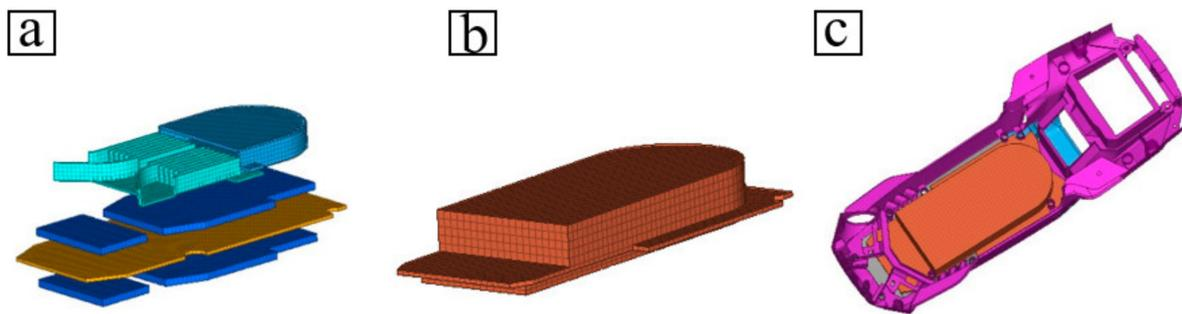
**Figure 11.** (a) Circuit board full-size model. (b) Circuit board simplified model. (c) Simplified model-4.
