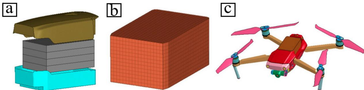
**Figure 8.** (a) Battery full-size model. (b) Battery simplified model. (c) Simplified model-1.
