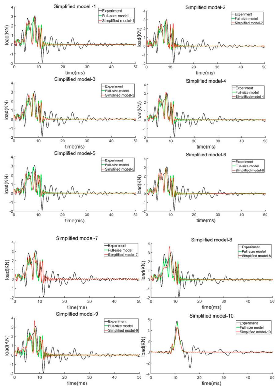
Figure 15. Comparison of impact loads in single simplified model.
