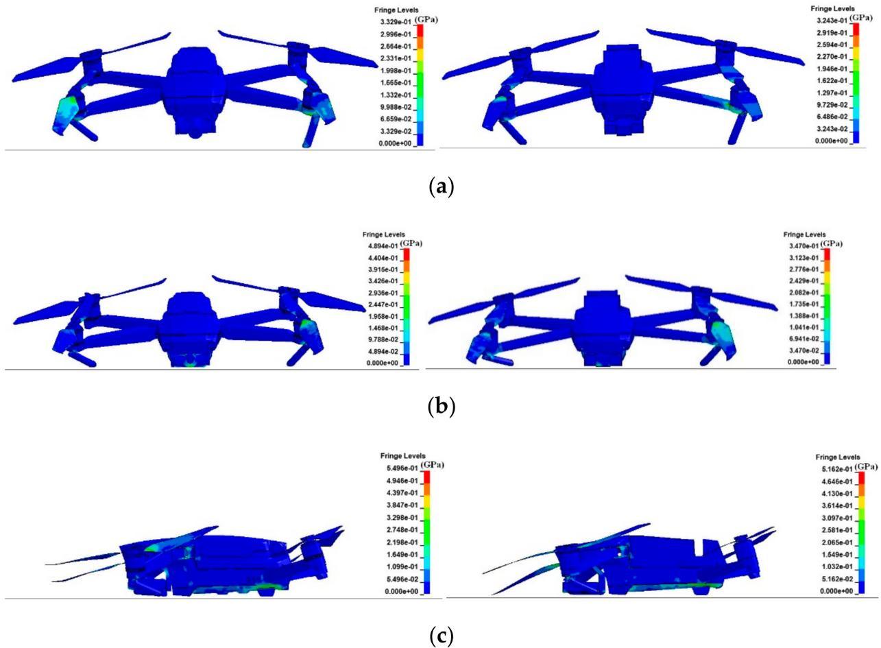
**Figure 20.** Comparison of stress distribution between the simplified model and the full-scale model at the typical time of the complete machine positive posture drop test. (a)  $2 \times 10^{-3}$  s time. (b)  $5 \times 10^{-3}$  s time. (c)  $8 \times 10^{-3}$  s time.
