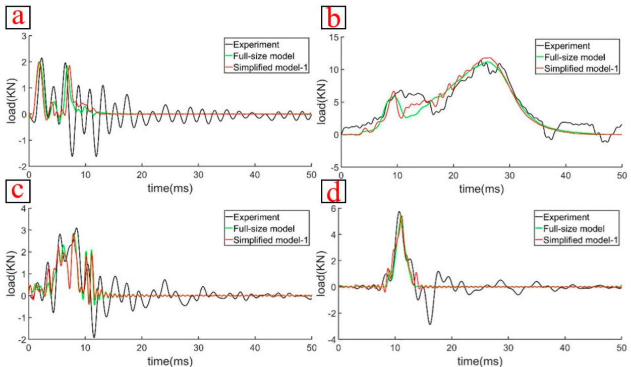
**Figure 19.** Peak load and error of combined simplified model. (a) Drop test of drone components. (b) Drop-weight test of drone components. (c) Drop test of drone positive posture. (d) Drop test of drone vertical posture.
