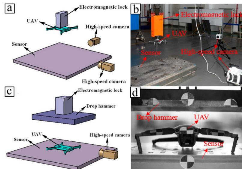
**Figure 3.** (a) Schematic diagram of drop test. (b) Drop test layout. (c) Schematic diagram of drop-weight test. (d) Drop-weight test layout.
