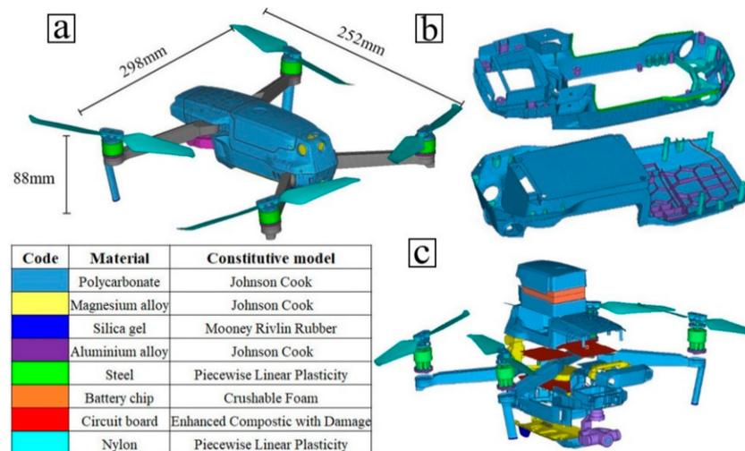
**Figure 1.** (a) Drone size. (b) Internal structure. (c) Drone materials.
