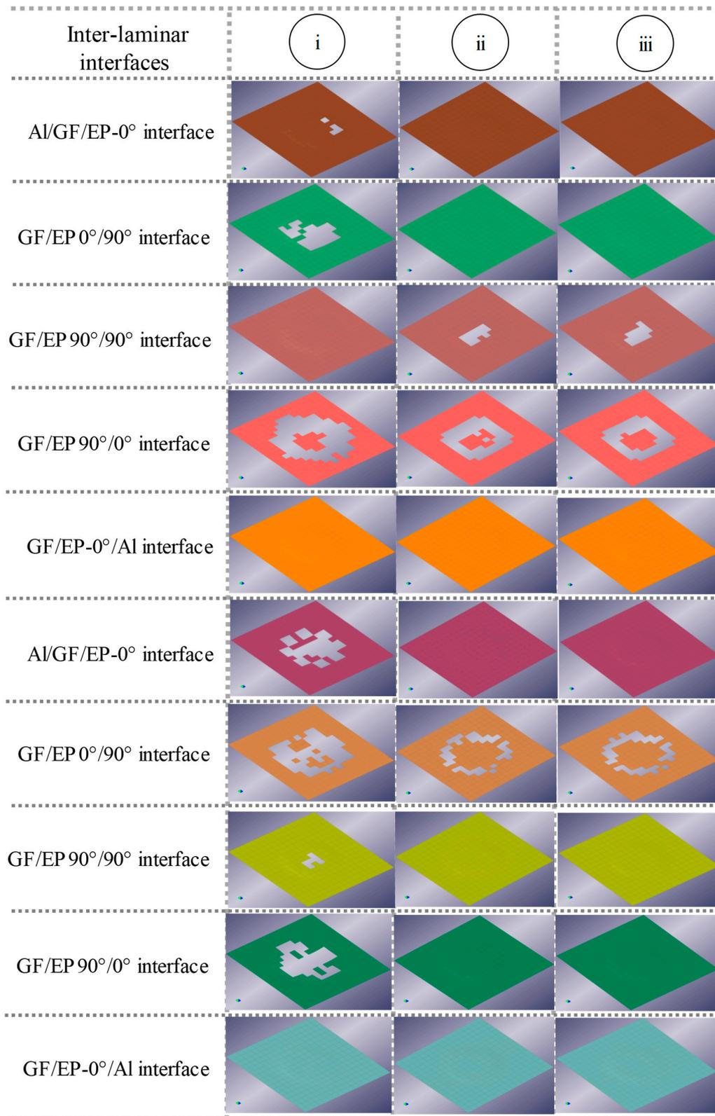
**Figure 9.** Debonding and delamination of cohesive interfaces of the GLARE laminate (i) at room temperature, (ii) at 80 °C (39% tougher epoxy-FM94), and (iii) at 80 °C (45% tougher epoxy-FM94) at 0.12 ms; the cohesive interfaces are organized from the impacted (top) to the non-impacted (bottom) side.
