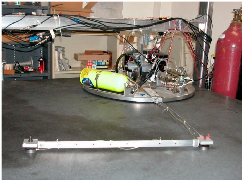
**Figure 1.** Flexible spacecraft robotic arm (very lightweight) attached to a rotational hub free-floating on planar air-bearing. The flexible arm is modeled using the lumped-mass technique where arm mass is distributed to discretized nodes as depicted in Figure 2.
