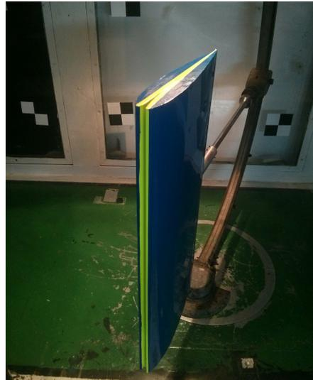
**Figure 22.** G2A30.7 wing segment fixed to the test apparatus during wind tunnel test.
