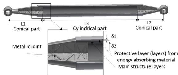
**Figure 6.** Main elements of the metal-composite rod.
