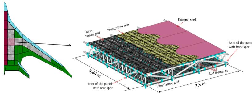
Figure 4. Double-lattice flat pressurized panel.
