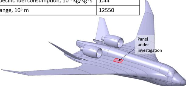
**Figure 2.** One of the prospective blended wing-body (BWB) configurations.
