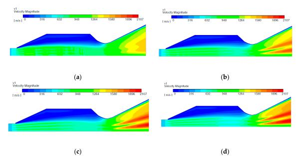
**Figure 14.** (**a**) Velocity contour for equivalence ratio of 0.4, (**b**) Velocity contour for equivalence ratio of 0.6, (**c**) Velocity contour for equivalence ratio of 0.8, (**d**) Velocity contour for equivalence ratio of 1.0.
