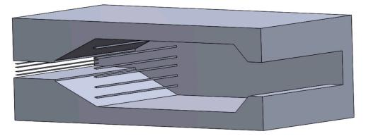
Figure 7. 3D view of dual-mode rectangular combustion chamber.
