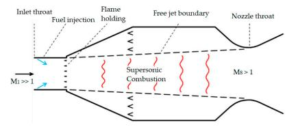
Figure 4. Free-jet dual-mode combustor in supersonic mode.
