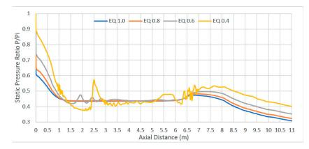
Figure 19. Variation of pressure with axial distance.
