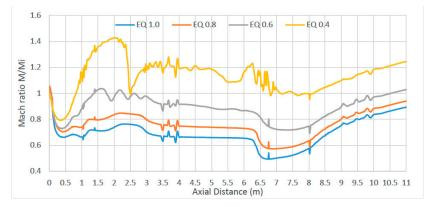
Figure 13. Variation of Mach ratio with axial distance.
