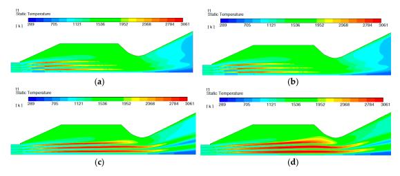
**Figure 17.** (a) Temperature contour for equivalence ratio of 0.4, (b) temperature contour for equivalence ratio of 0.6, (c) temperature contour for equivalence ratio of 0.8, (d) temperature contour for equivalence ratio of 1.0.
