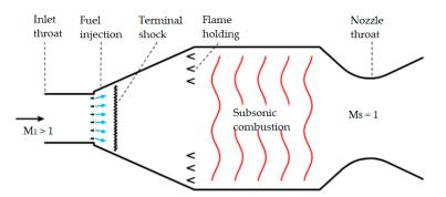
Figure 3. Free-jet dual-mode combustor in subsonic mode.
