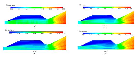
**Figure 12.** (a) Mach number contour for equivalence ratio of 0.4, (b) Mach number contour for equivalence ratio of 0.6, (c) Mach number contour for equivalence ratio of 0.8, (d) Mach number contour for equivalence ratio of 1.0.
