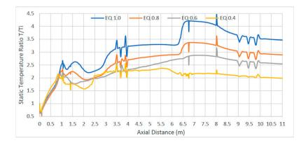
Figure 16. Variation of temperature with axial distance.
