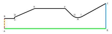
Figure 5. Combustion chamber geometry.
