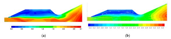
Figure 10. Comparison of Mach contour; (a) computational result, (b) experimental result [17].
