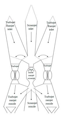
Figure 2. Engine configuration.
