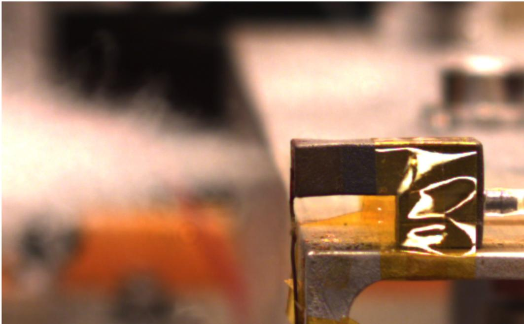
**Figure 17.** A photograph of the thruster system operating during the plume temperature measurement experiment. Condensation surrounding the plume is visible.
