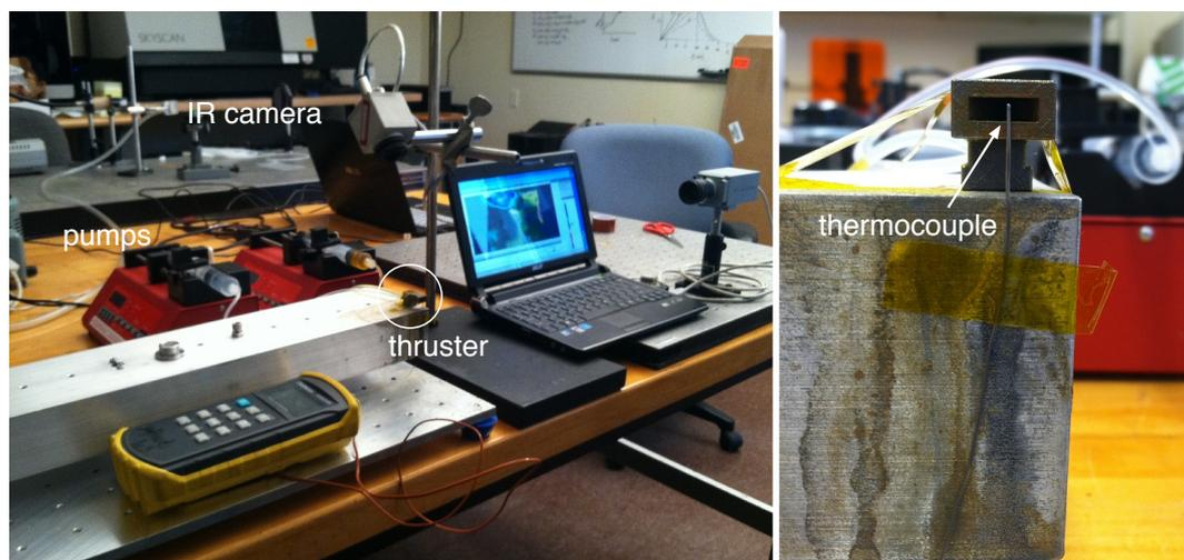
**Figure 12.** (Right) Photograph of DMLS stainless steel nozzle used for plume temperature measurement. A type K thermocouple was placed directly in the center of the nozzle exit for temperature measurements. (Left) Photograph of entire experimental set-up including thermal imaging camera, video camera, and digital thermometer.
