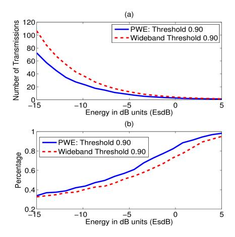
Figure 6. (a) ANI vs. transmit energy  $(E_s)$  in dB  $(E_s dB)$  for PWE and wideband waveforms and (b)  $P_{cd}$  vs. transmit energy  $(E_s)$  in dB (EsdB) for PWE and wideband waveforms using a probability threshold of 0.90 with the SHT-CRr platform.
