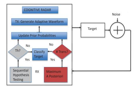
**Figure 1.** Block diagram of sequential hypothesis testing (SHT)-cognitive radar (CRr) and MAP-CRr for target recognition or identification application.
