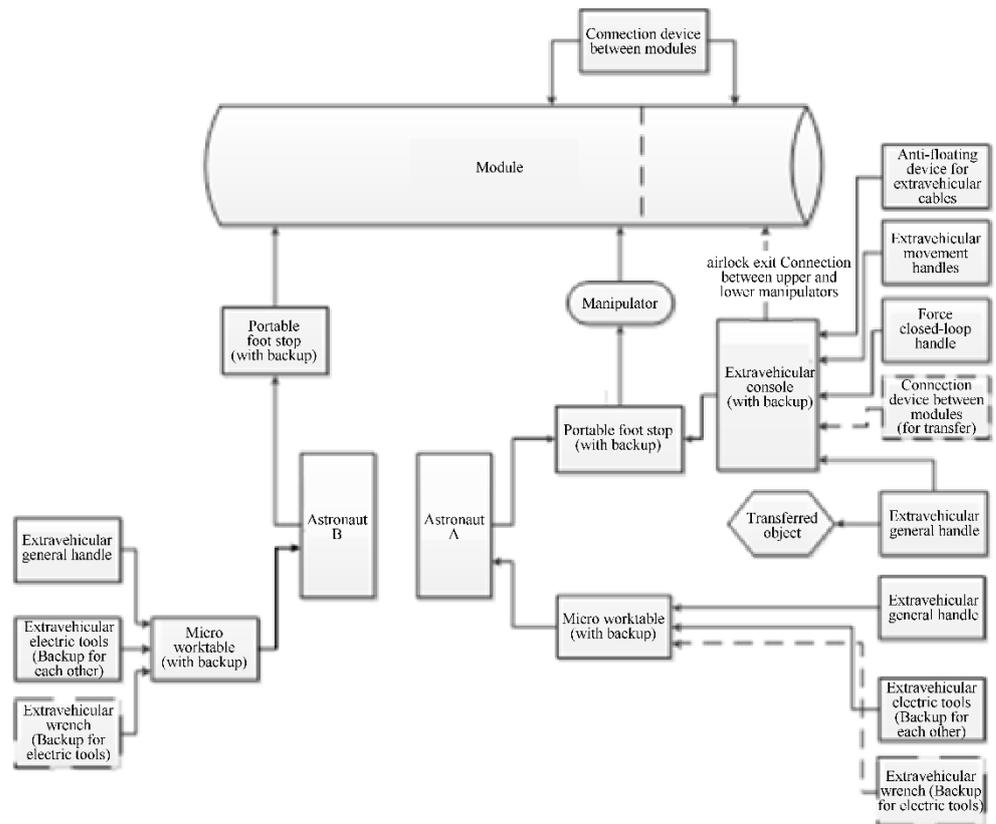
Figure 18. Combined application of general facilities in the space station.
