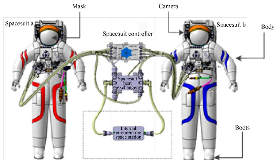
**Figure 23.** Connection between extravehicular spacesuits and on-board support devices.
