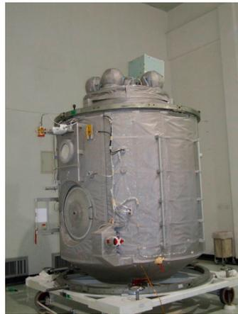
**Figure 1.** Overall structure of the airlock module in Shenzhou VII.
