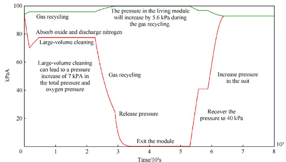
**Figure 9.** Pressure curve in the module during the EVA process.
