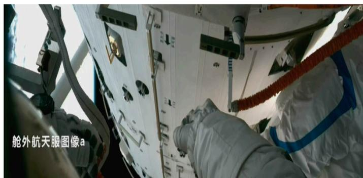
**Figure 15.** Transfer handrail on the module's surface.
