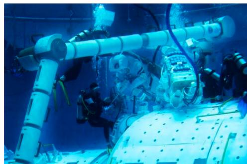
**Figure 32.** Verification of the operation of manipulators used by astronauts under water.
