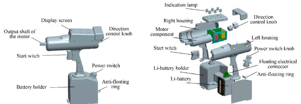
**Figure 19.** Structure of extravehicular electric tools.
