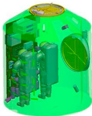
**Figure 6.** Space simulation of the airlock module.
