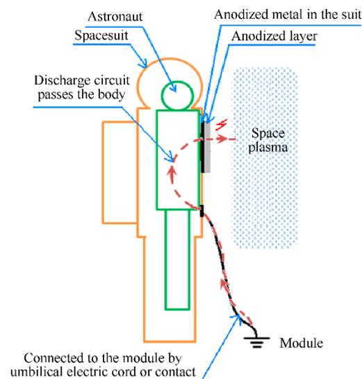
**Figure 29.** Discharge circuit of the extravehicular spacesuits.
