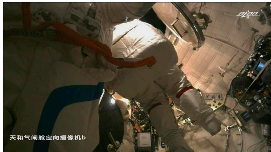
**Figure 7.** An astronaut was opening the module door by using the driving handle.
