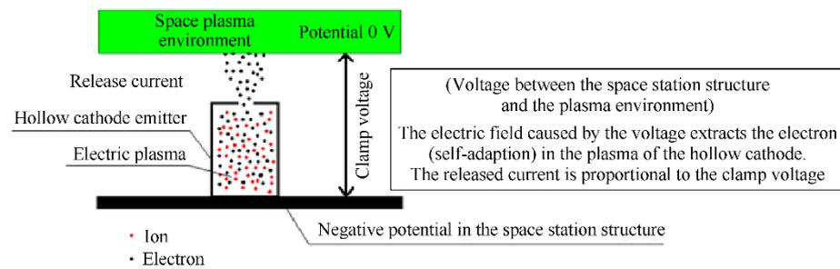
**Figure 30.** Discharge circuit of the extravehicular spacesuit.
