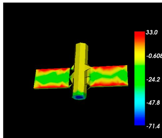
**Figure 28.** Simulation of the surface potential of the core module.
