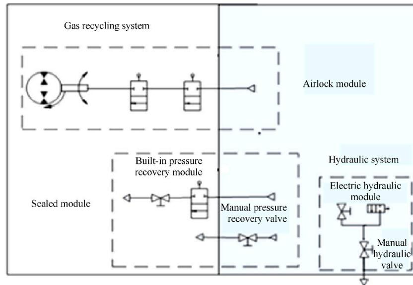
**Figure 8.** Composition of the pressure relief/recovery system in the airlock module.
