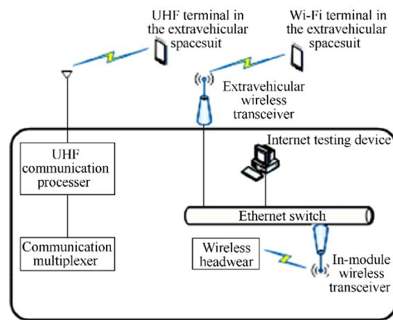
**Figure 24.** Connection between extravehicular spacesuits and on-board support devices.
