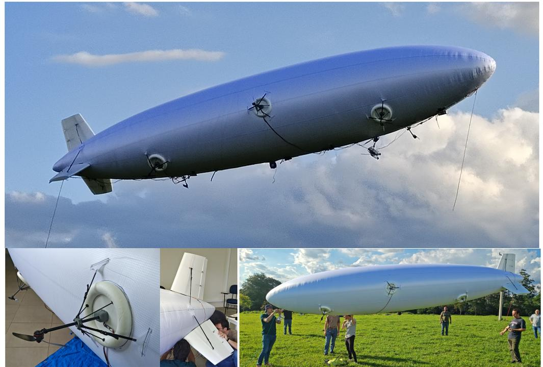
**Figure 1.** The Noamini airship in the maiden flight in Brazil. Bottom: the inverted-Y tail and the tilting propeller, which is rotated by a servo in its base.
