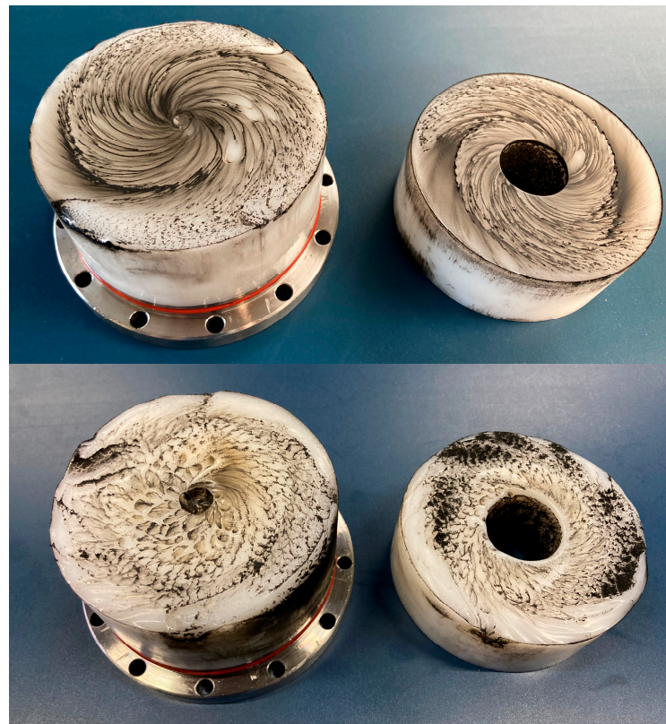
Figure 12. Fuel grains after successful burn showing the vortex pattern on their surfaces. Test 1 ( up ), Test 3 ( bottom ).
