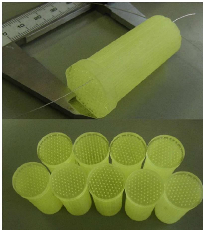
**Figure 27.** Fuel grains made from 80–90% acrylic acid ester, 5% hexamethylene acrylate, and a photopolymerization initiator. Image reprinted from Ref. [62] with permission from AIAA.
