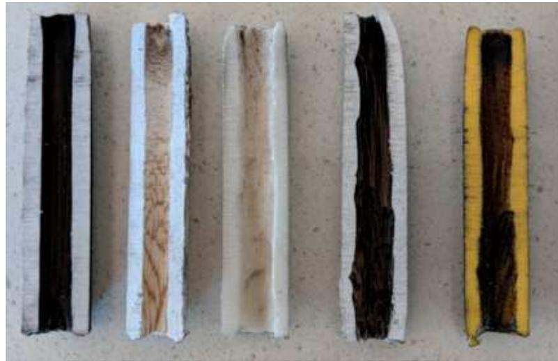
**Figure 7.** Cross section of the small-scale fuel grains after firing, left to right: ABS, PLA, PP, ASA, and PTEG. Image reprinted from Ref. [22] with permission under the Creative Commons 4.0 License.
