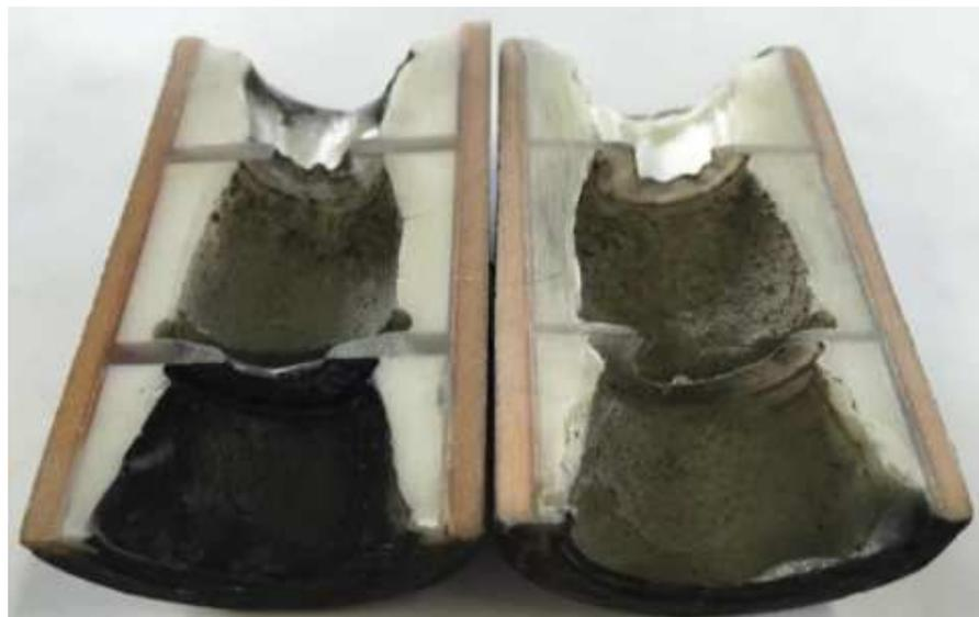
**Figure 22.** Comparison of 0.100" diaphragm (left) and 0.050" diaphragm (right). Image reprinted from Ref. [28] courtesy of and by permission of the Aerospace Corporation.
