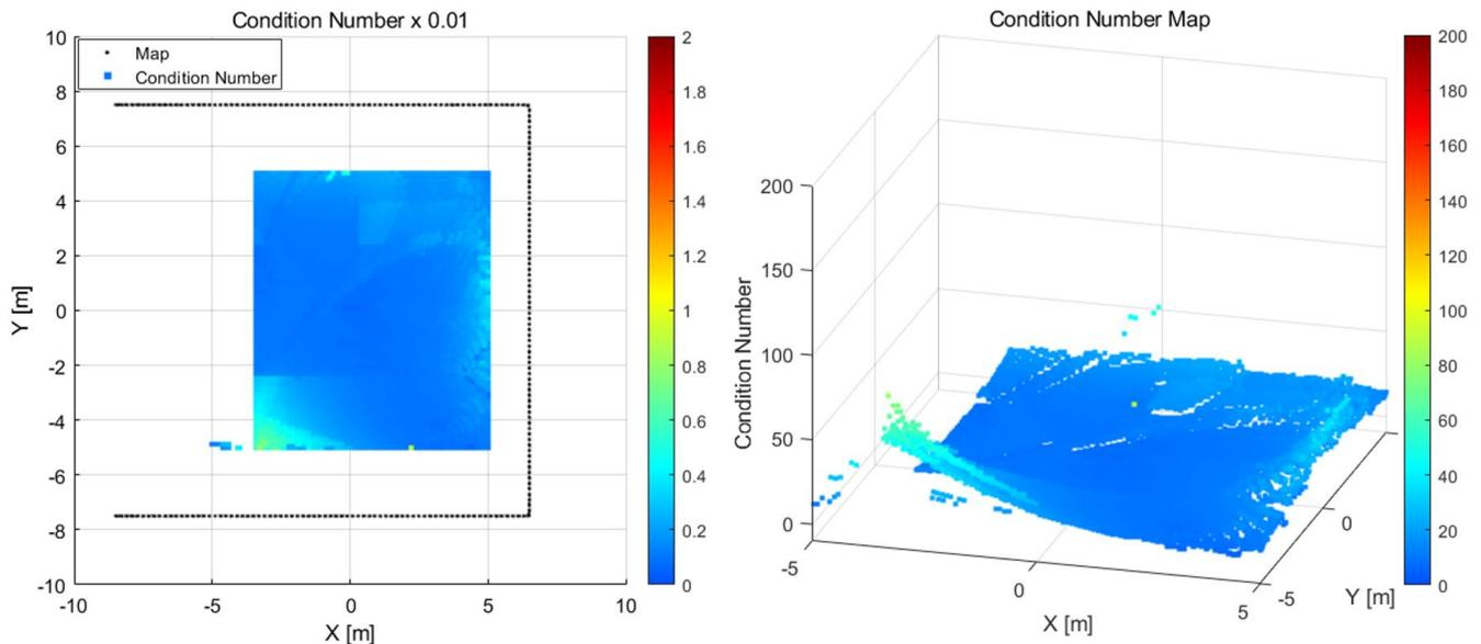
**Figure 5.** Condition number map in an environment where the left side is open and three sides are closed.
