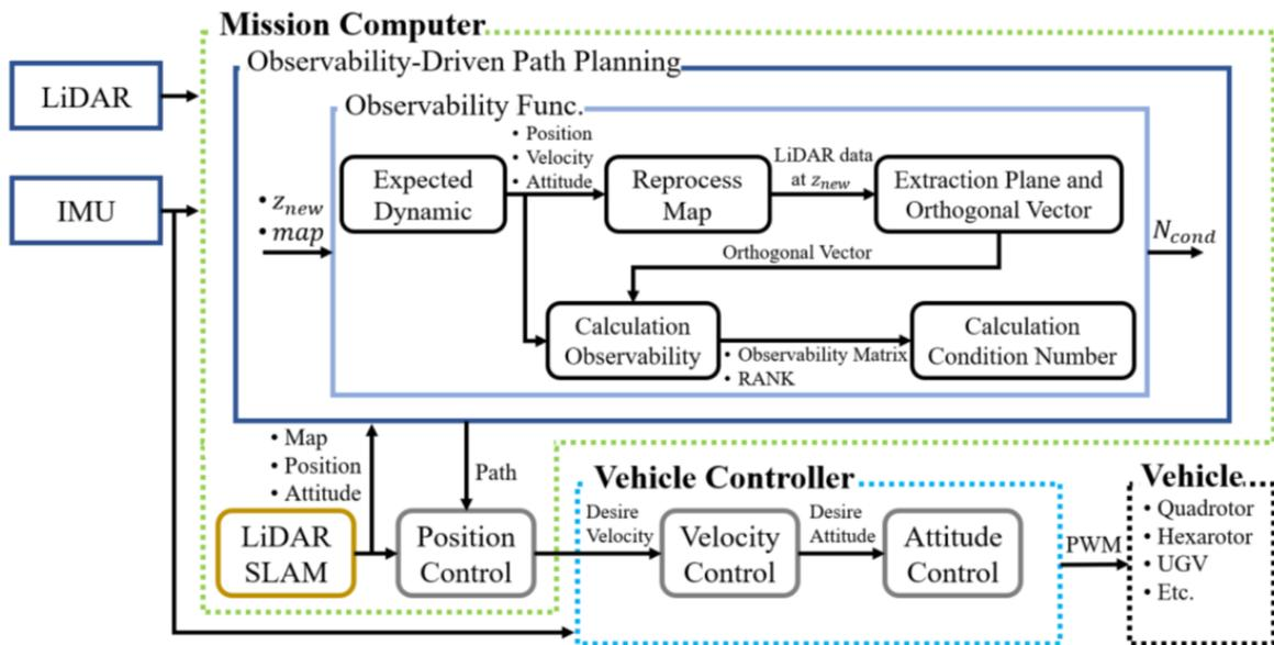
Figure 11. Test platform schematic diagram. Green dotted line: mission computer composed of NUC. Blue dotted line: vehicle controller based on Cortex-M4. Black dotted line: actuator hardware.
