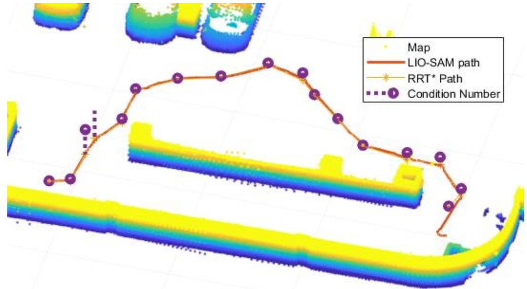
**Figure 14.** Tree of path planning algorithm in the experimental environment.
