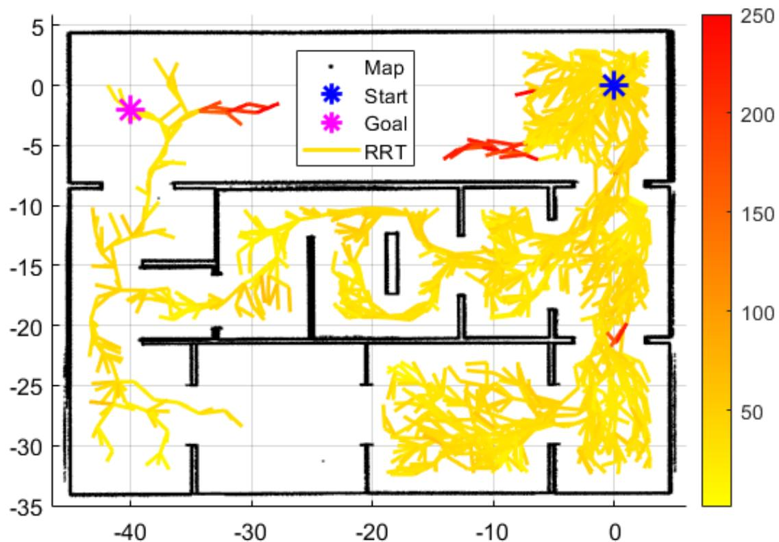
**Figure 9.** Tree of path planning algorithm in the maze environment. The blue dot is the starting point, the magenta dot is the destination, and the black dot is the point cloud map. The line represents the ODPP tree, and the color varies according to the condition number. Higher values are shown in red, and lower values are in yellow.
