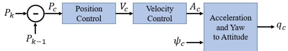
**Figure 2.** Velocity and attitude prediction controller structure.
