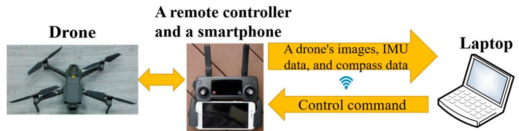
**Figure 2.** Hardware architecture of the proposed ADES.
