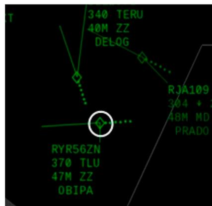
**Figure 3.** Radar track highlight following callsign detection (Captured from Supplementary Materials).
