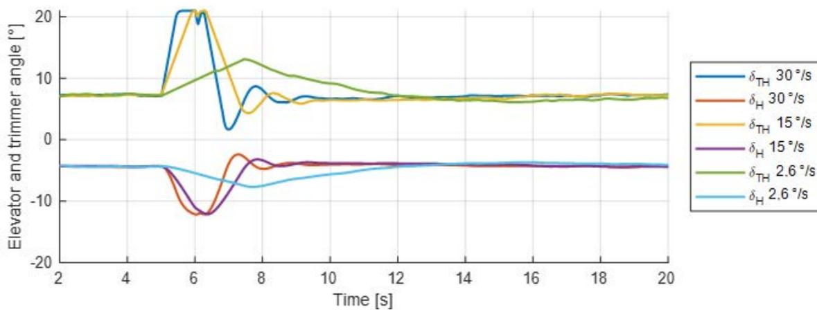
Figure 10. Elevator and trimmer angles during stabilisation after disturbance in the longitudinal channel.
