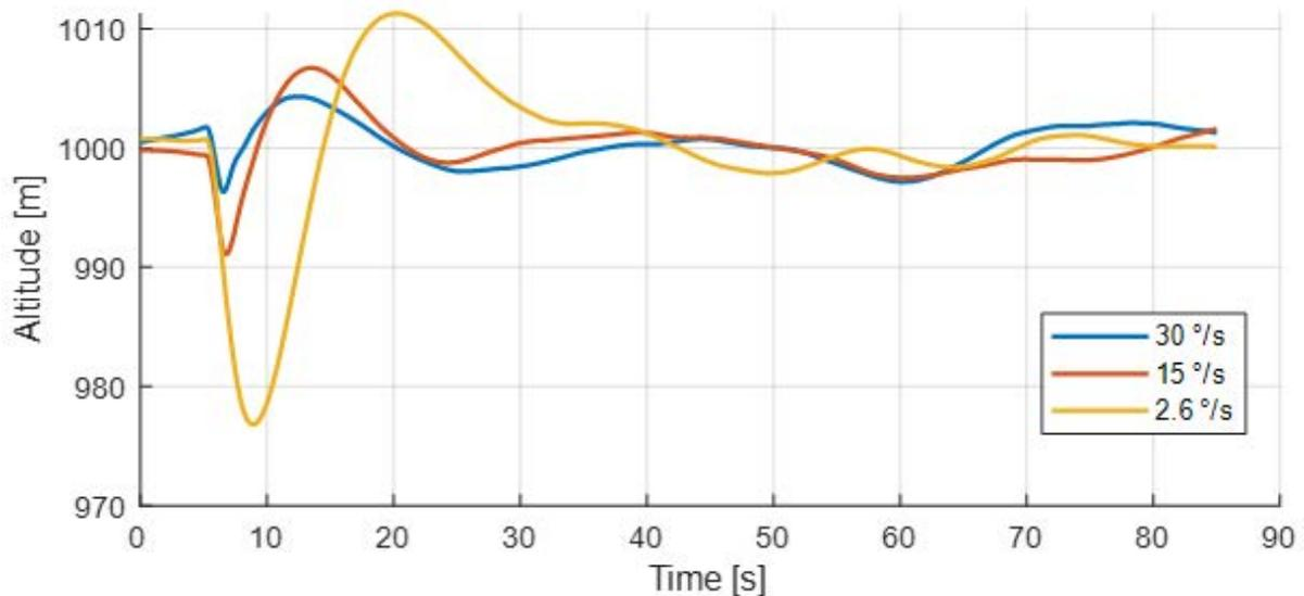
**Figure 8.** Altitude stabilisation after disturbance in the longitudinal channel.
