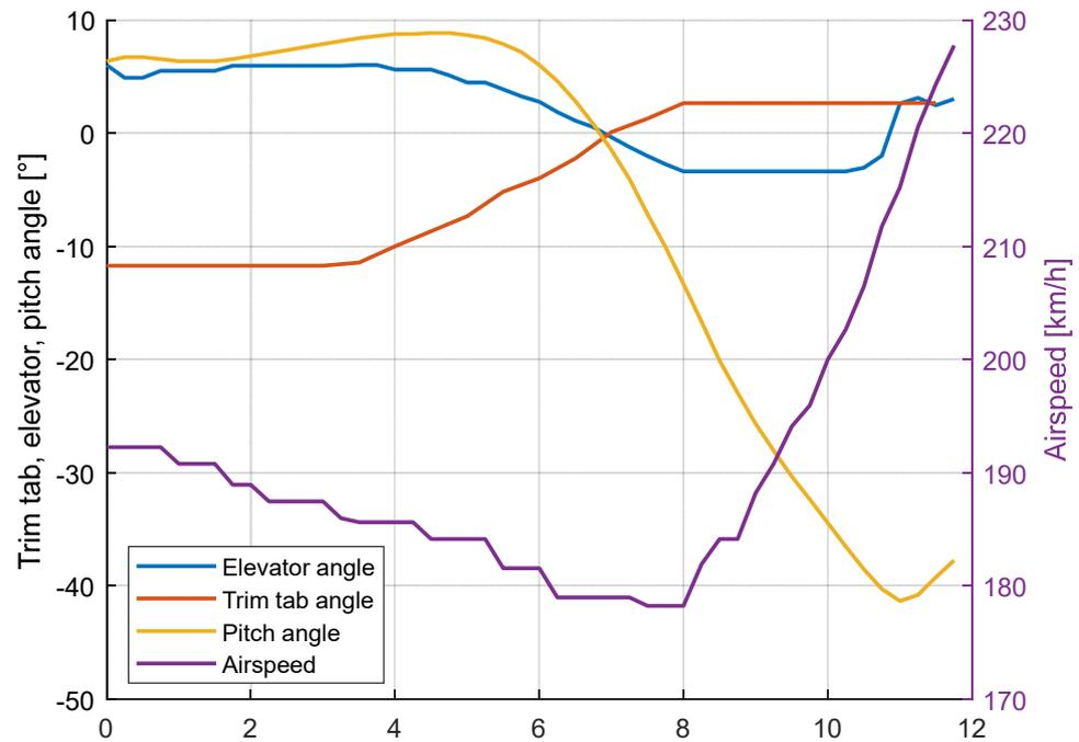
Figure 4. Flight test results of elevator trimmer movement to an extreme position.
