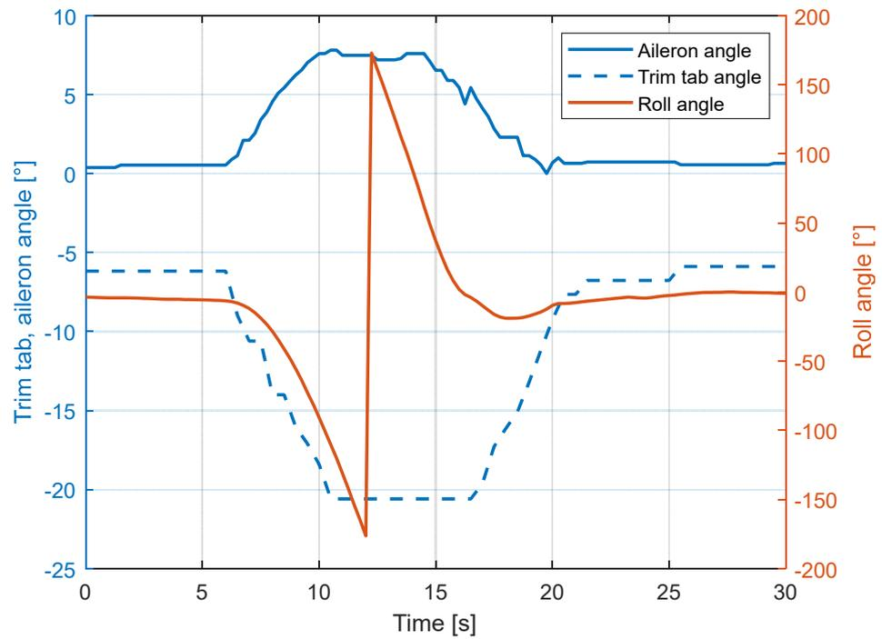
**Figure 2.** Flight test results during trim-tab-only manually controlled flight—barrel roll manoeuvre.
