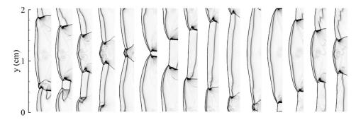
**Figure 12.** Density gradient of the detonation front from x = -56.25 to x = -59.625.
