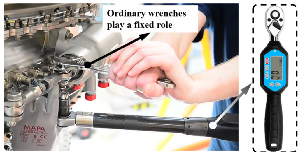
Figure 18. Schematic diagram of a constant-torque wrench [89,90].
