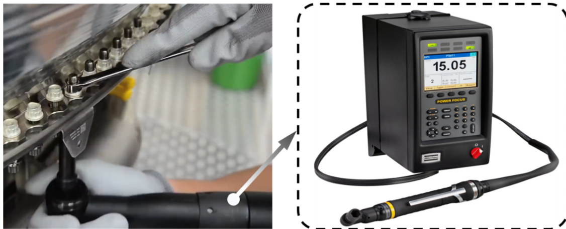
Figure 19. Schematic diagram of an electric wrench.
