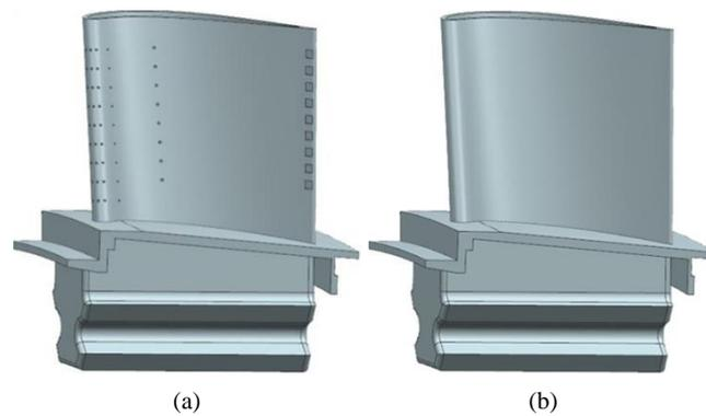
**Figure 10.** Detail features of blade geometric model suppression: (a) Before suppression, (b) After suppression.
