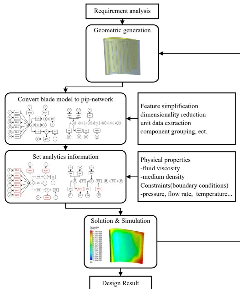
Figure 1. Diagram of the blade’s PNC.
