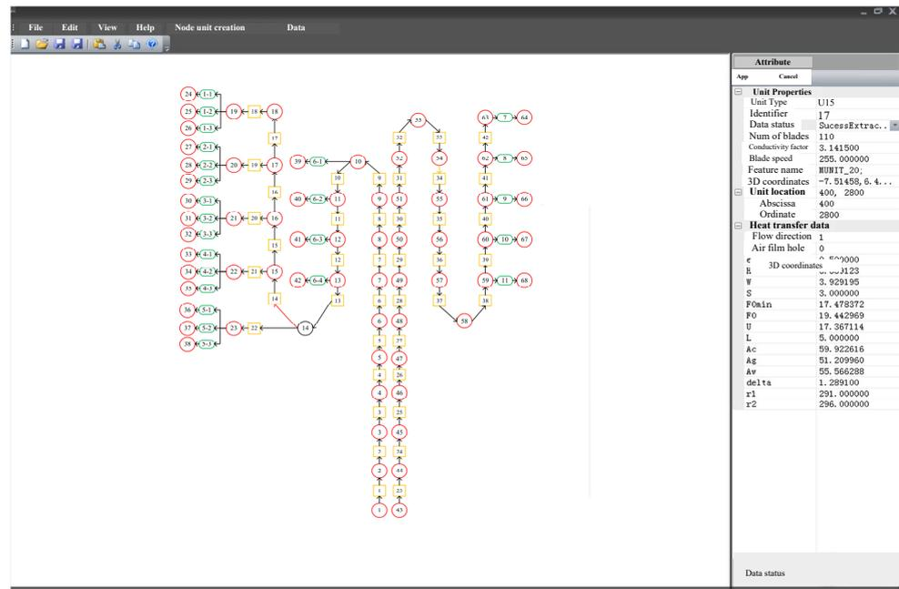
Figure 35. Pipe network drawing interface.
