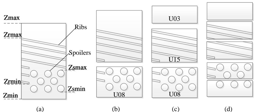
**Figure 20.** Schematic diagram of diameter division process: (a) longitudinal flow channel, (b) U08 unit separation, (c) U15 unit separation, and (d) internal division of similar units.
