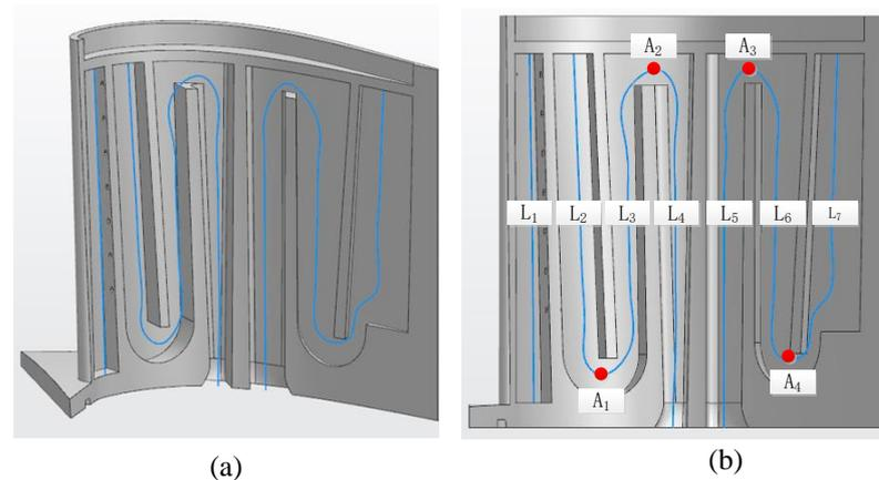
**Figure 11.** Skeleton line adaptive division method: (a) Extraction of skeleton lines imitating fluid flow. (b) Result of skeleton lines adaptive division.
