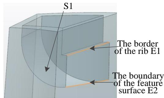
Figure 17. Schematic diagram of characteristic boundary of turning section.
