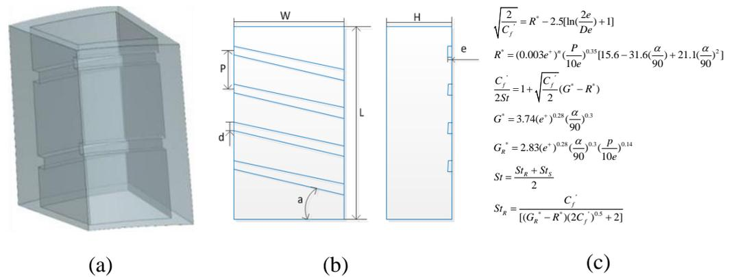
**Figure 15.** Schematic diagram of of main flowing unit calculation: (a) Main flowing unit model. (b) Geometric design parameters. (c) Extracted data formula [33].
