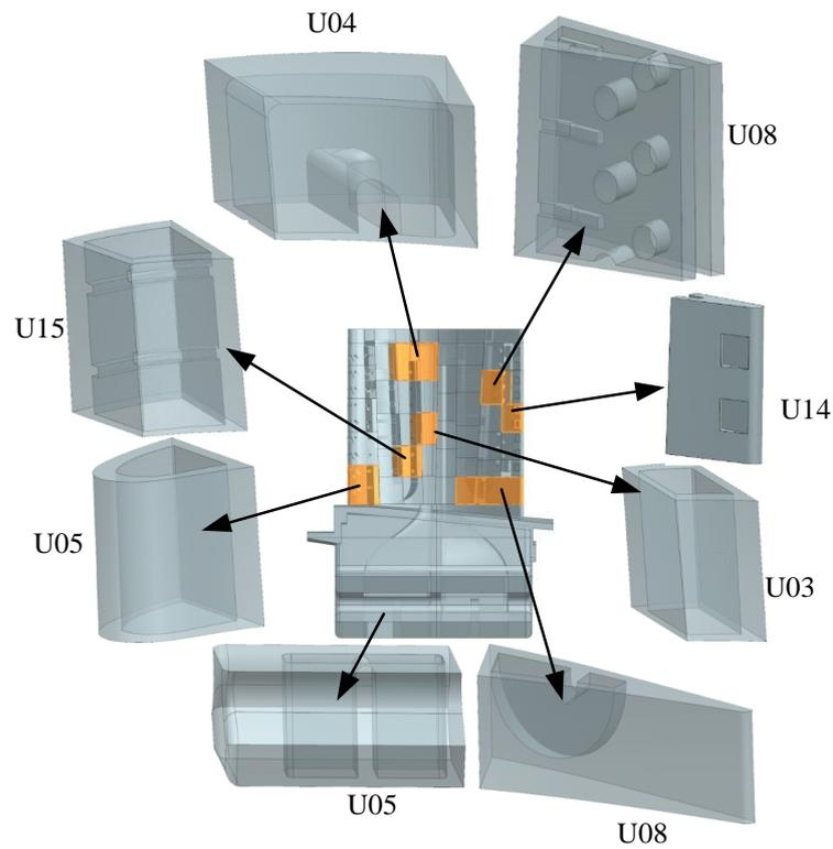
Figure 21. Adaptive division results of one blade model.
