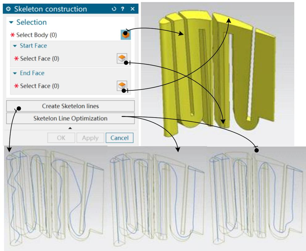
Figure 31. Interface of skeleton line of the flow path.
