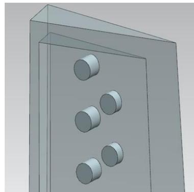
Figure 18. Schematic diagram of the cooling structure of the spoiler column.
