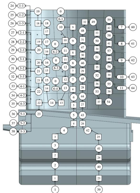
**Figure 25.** Topological model diagram of blade flow channel.
