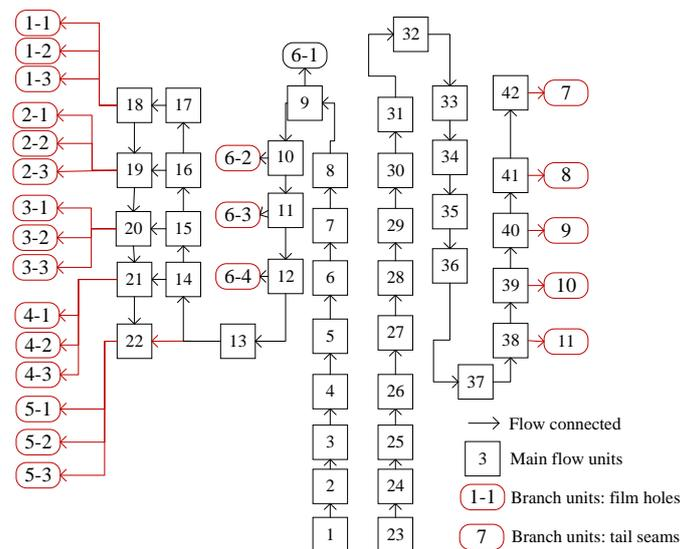
Figure 24. The connection relationships between the flow units of blade.
