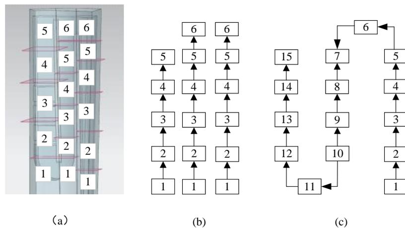
Figure 22. Connection relationship of the main flow channel units: (a) main channel units, (b) segmented flow channel unit connectivity, and (c) combination of multi-stage flow channel relationship.
