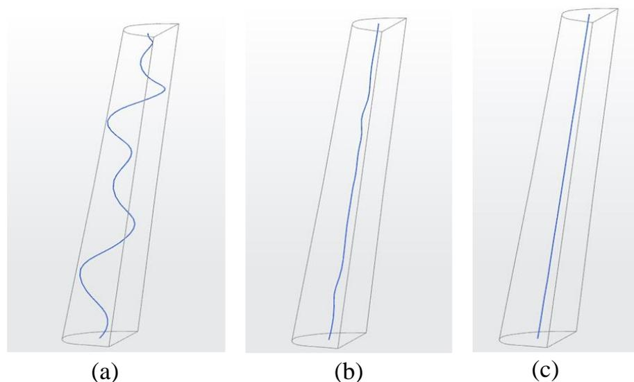
**Figure 8.** Iterative optimization results of the single-channel flow path skeleton line: (a) Original flow path skeleton line; (b) Skeleton line obtained by one iteration; (c) Final optimized skeleton line.
