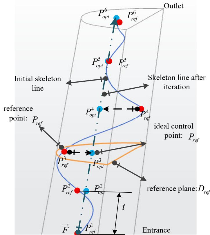
**Figure 6.** Basic idea of iterative optimization of the skeleton line.
