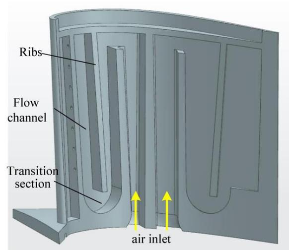
**Figure 9.** Illustration of turbine blade spacer ribs.
