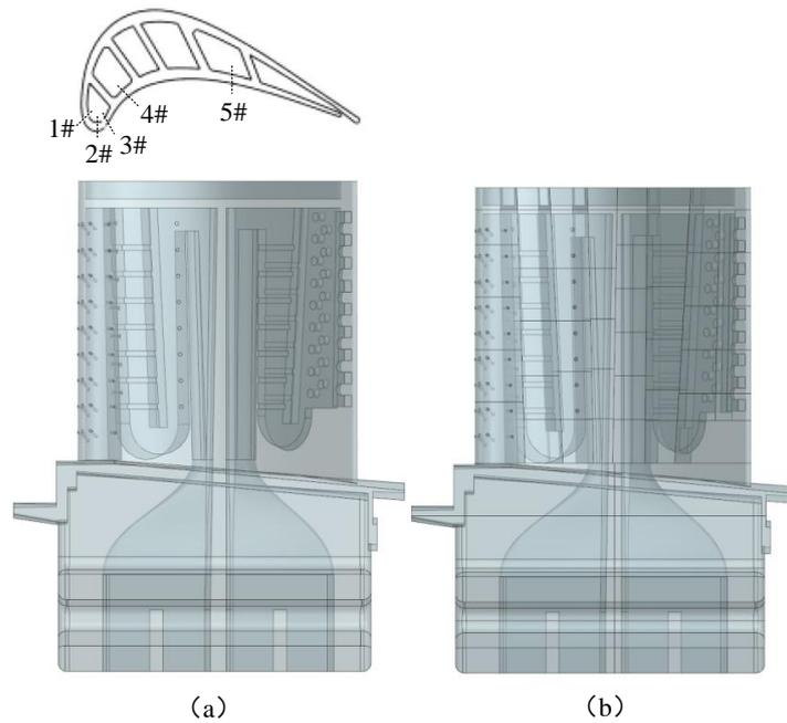
Figure 34. Blade model and division: (a) The blade 3D geometric model; and (b) the blade 3D geometric model after adaptive division.
