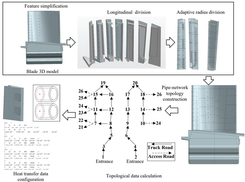
Figure 2. Process and scheme of extracting heat transfer data for composite cooling blades.
