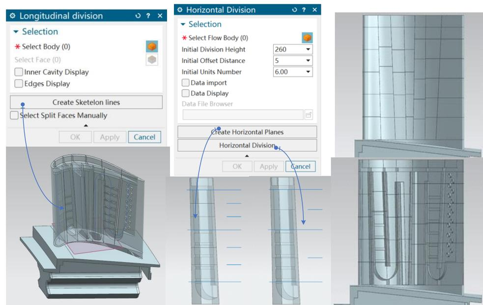
Figure 32. Interface of the adaptive division of flow units based on skeleton lines.
