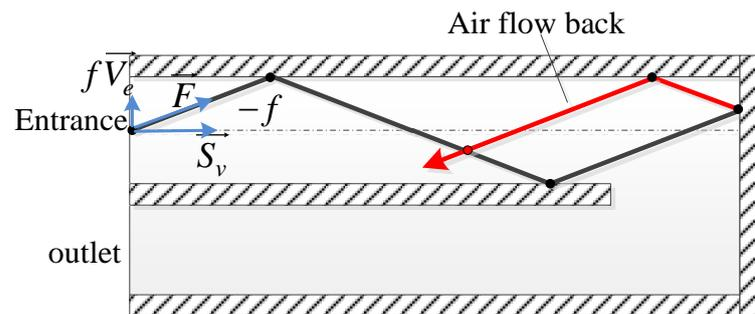
Figure 4. Inappropriate initial airflow direction causes airflow backflow.
