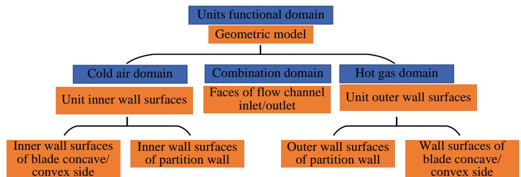
**Figure 28.** Blade functional and geometric domain decomposition.
