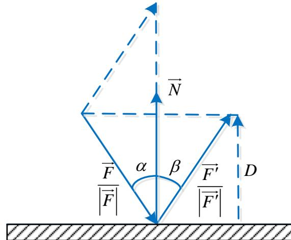
Figure 3. Schematic diagram of the assumption of air-flow wall reflection.
