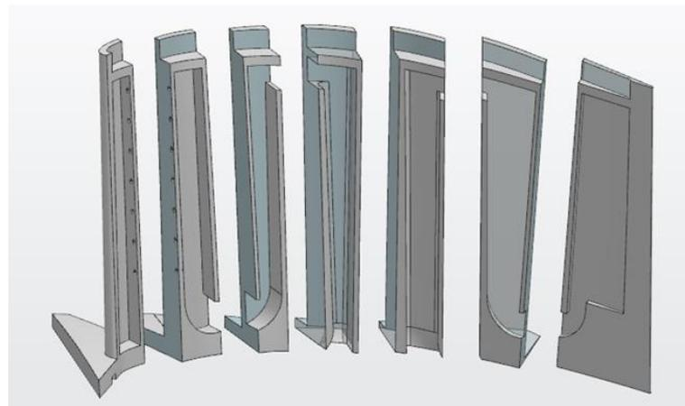
**Figure 13.** Adaptive longitudinal division results of the blade based on skeleton lines.
