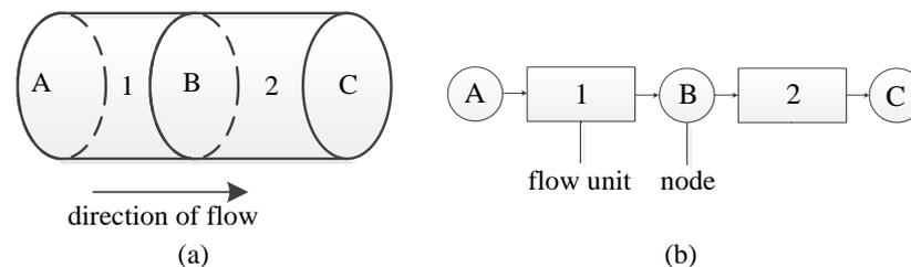
**Figure 14.** Calculation principle of flowing unit: (a) Schematic diagram of the divided flow channel. (b) Abstracted computing unit.
