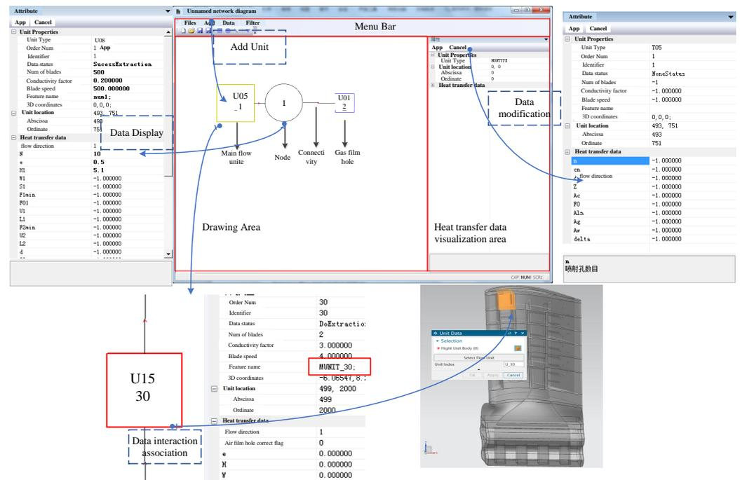
Figure 33. Network diagram visualization and data configuration.
