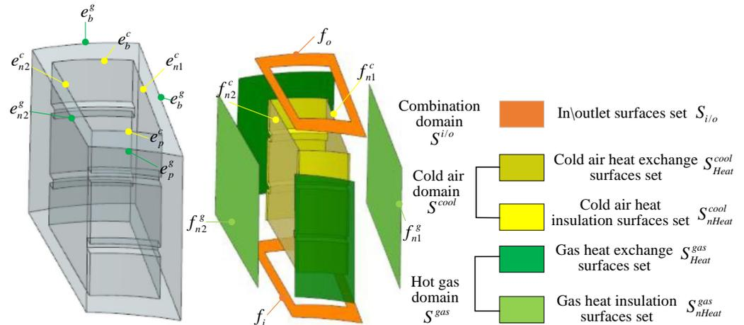
Figure 29. Spoiler fin unit geometric composition and functional decomposition.
