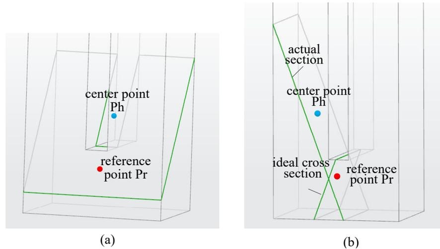
**Figure 7.** Schematic representation of iterative optimization criteria: (a) judgment of unevenness condition, and (b) judgment of distance condition.
