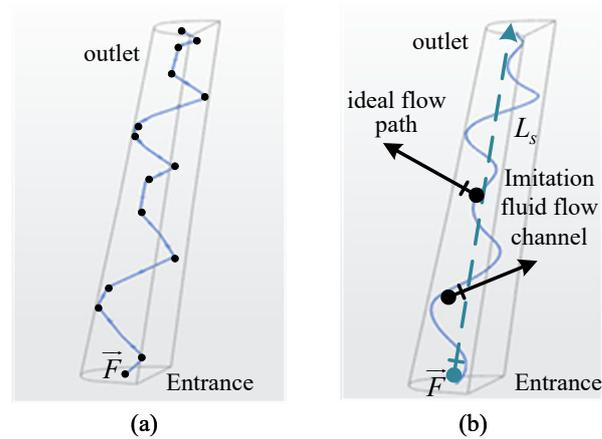
**Figure 5.** Schematic diagram of the initial reference pipe-network topology skeleton line for a single channel: (a) Flow collision simulation and control vertices, and (b) cubic spline fitting of the fluid flow path.
