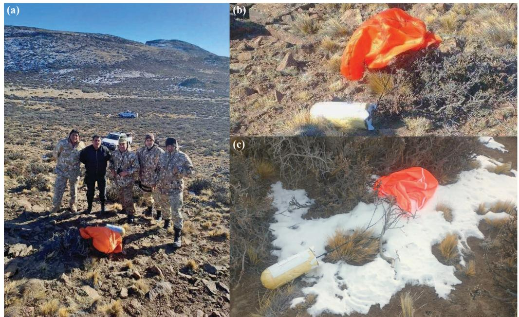
**Figure 7.** Landing sites of the DRS capsules in Argentina. (a) General terrain and the search and rescue team from the governor’s office of Santa Cruz Province. The bright-orange parachutes of DRS1 (b) and DRS2 (c) were visible from a distance. The white foam shell and release crown were finally also visible; the foam helped to insulate and waterproof DRS2 when it landed on snow.
