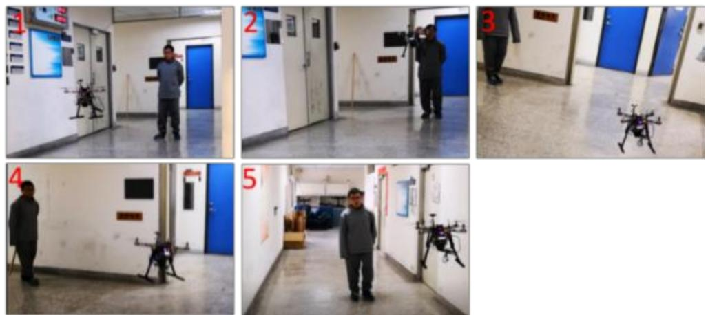
**Figure 23.** UAV tracking target test at the corridor (The sequence of target movement and UAV tracking is shown in 1–5).
